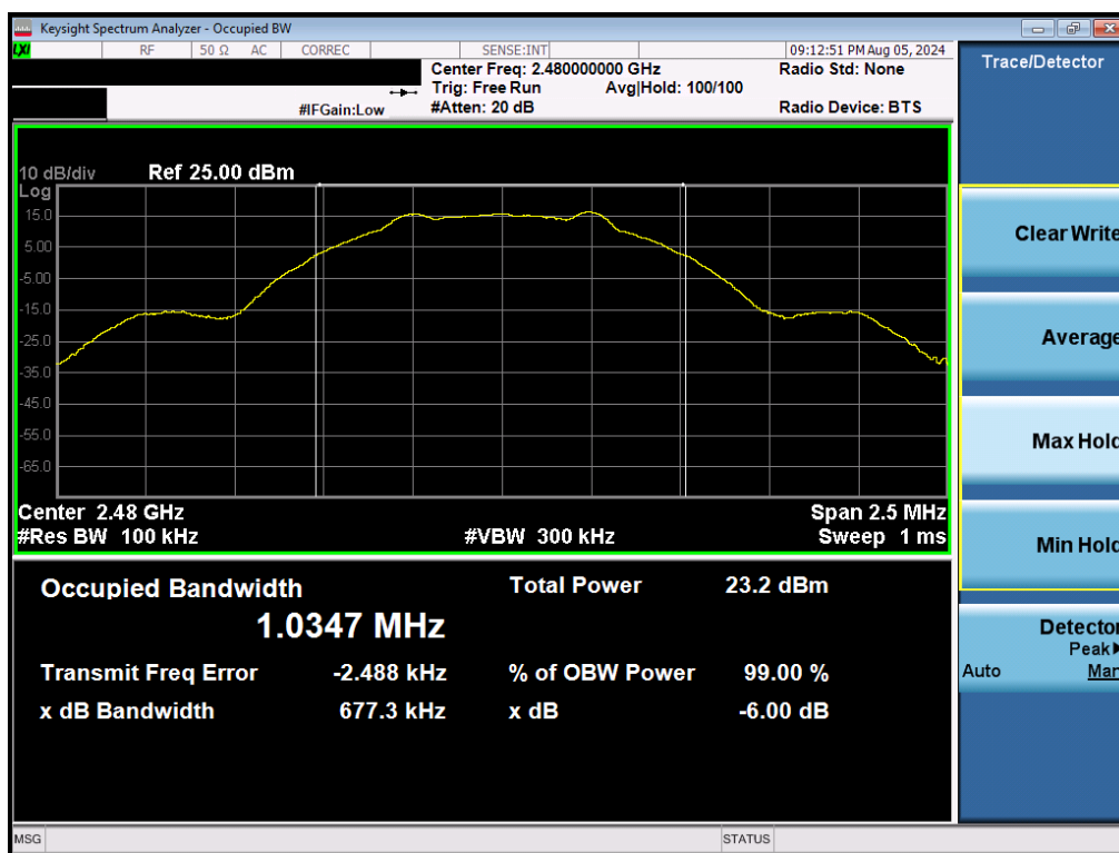
Plot 7-3. 6dB BW & 99% OBW Plot (Bluetooth (LE), 1Mbps – Ch. 39)
