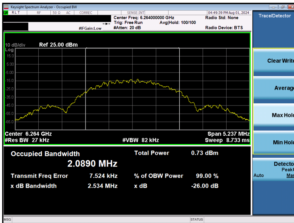
Plot 7-5. 26dB BW & 99% OBW (NB UNII LE, 2Mbps – 6264MHz)
