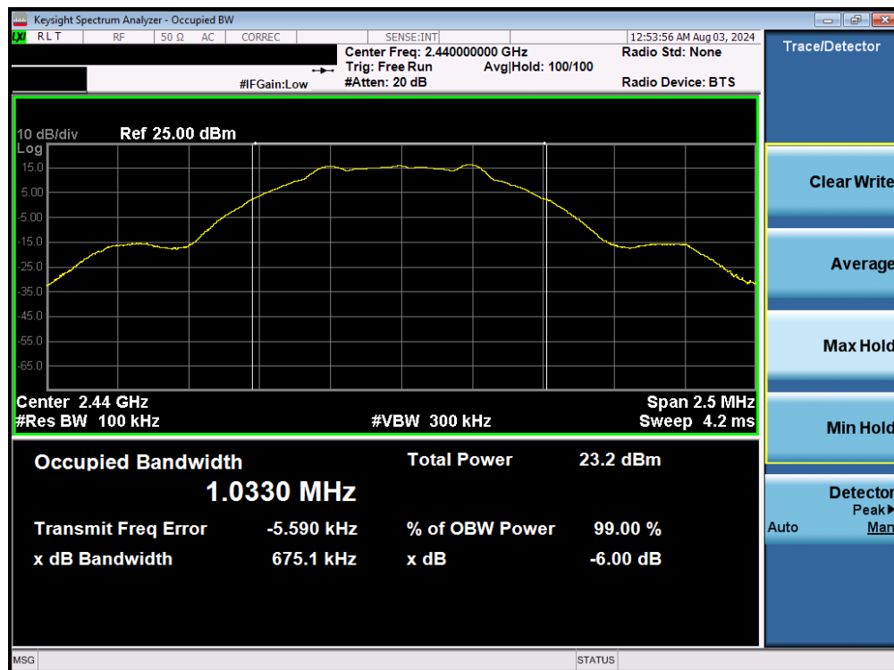
Plot 7-2. 6dB BW & 99% OBW Plot (Bluetooth (LE), 1Mbps, – Ch. 19)
