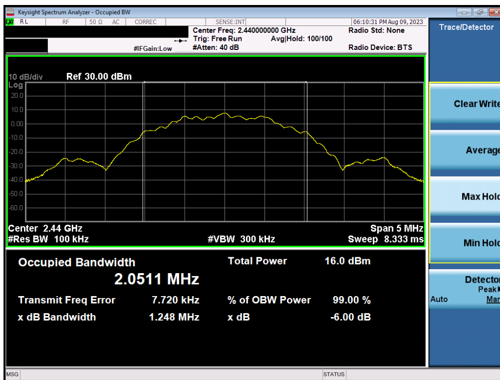
Plot 7-5. 6dB BW & 99% OBW Plot (Bluetooth (LE), 1Mbps – Ch. 19)
