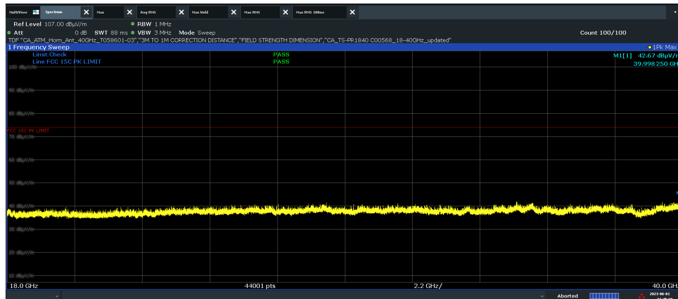
Plot 7-32. Radiated Spurious Emissions above 18GHz (BT GFSK – Ch. 78, Pol H)
