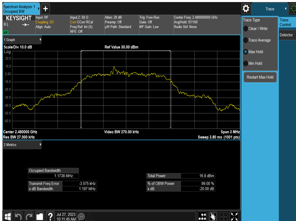
Plot 7-6. 20dB BW and 99% OBW Plot (Bluetooth, 8DPSK – Ch. 78)
