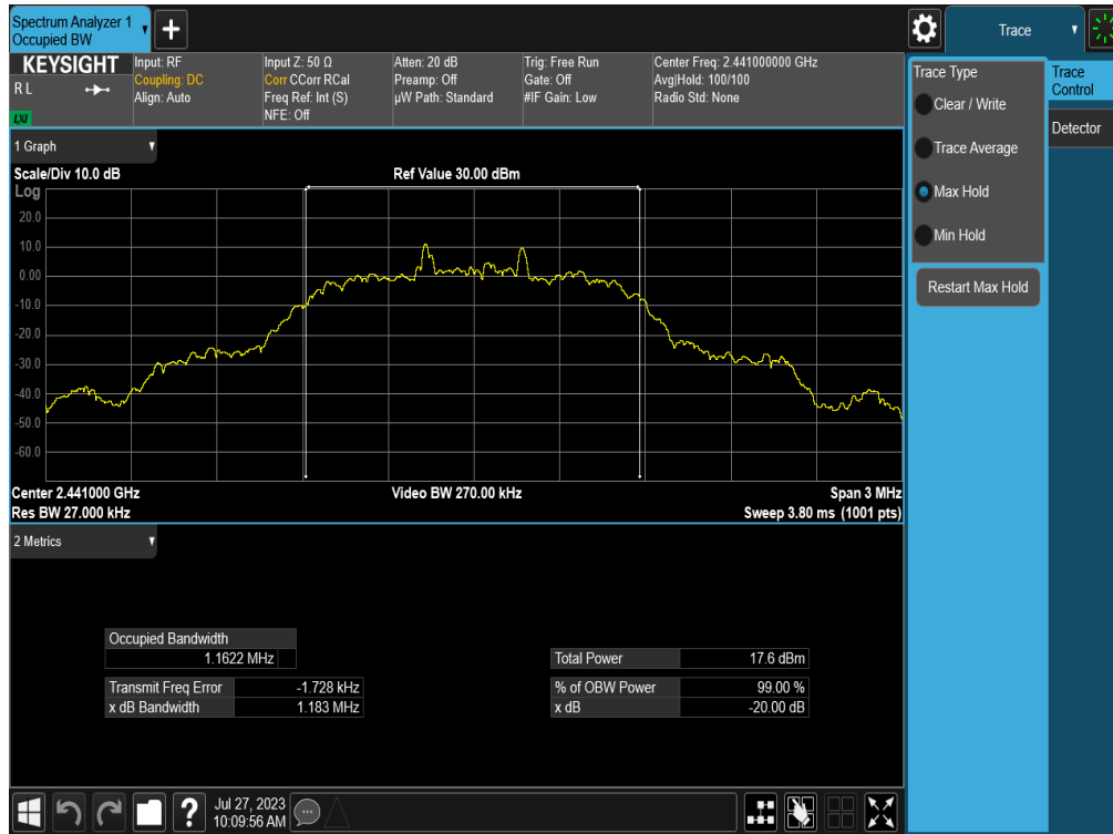
Plot 7-5. 20dB BW and 99% OBW Plot (Bluetooth, 8DPSK – Ch. 39)
