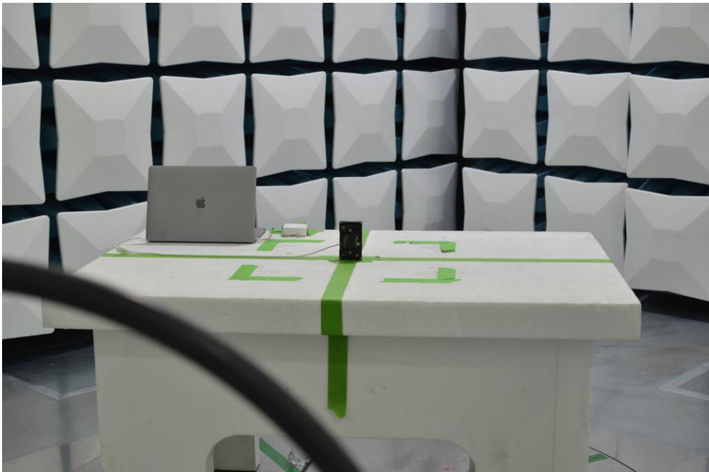
Figure 20: 9kHz-30MHz Test Setup (Front View)
