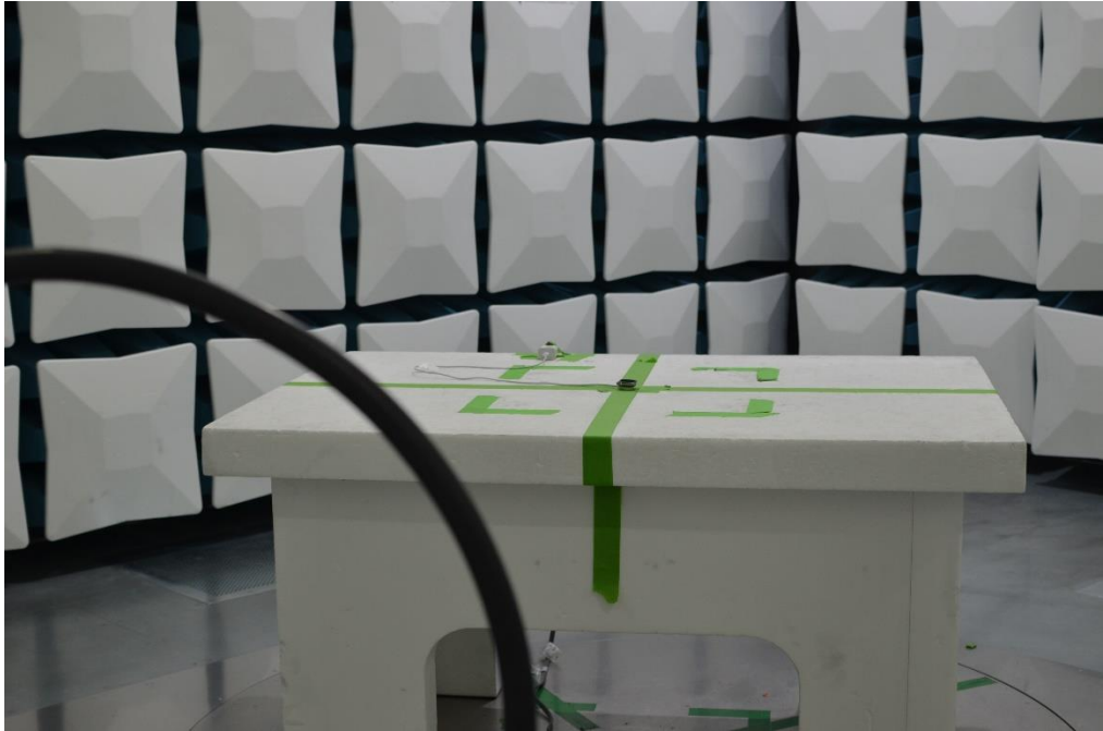
Figure 23: 9kHz-30MHz Test Setup (Front View)
