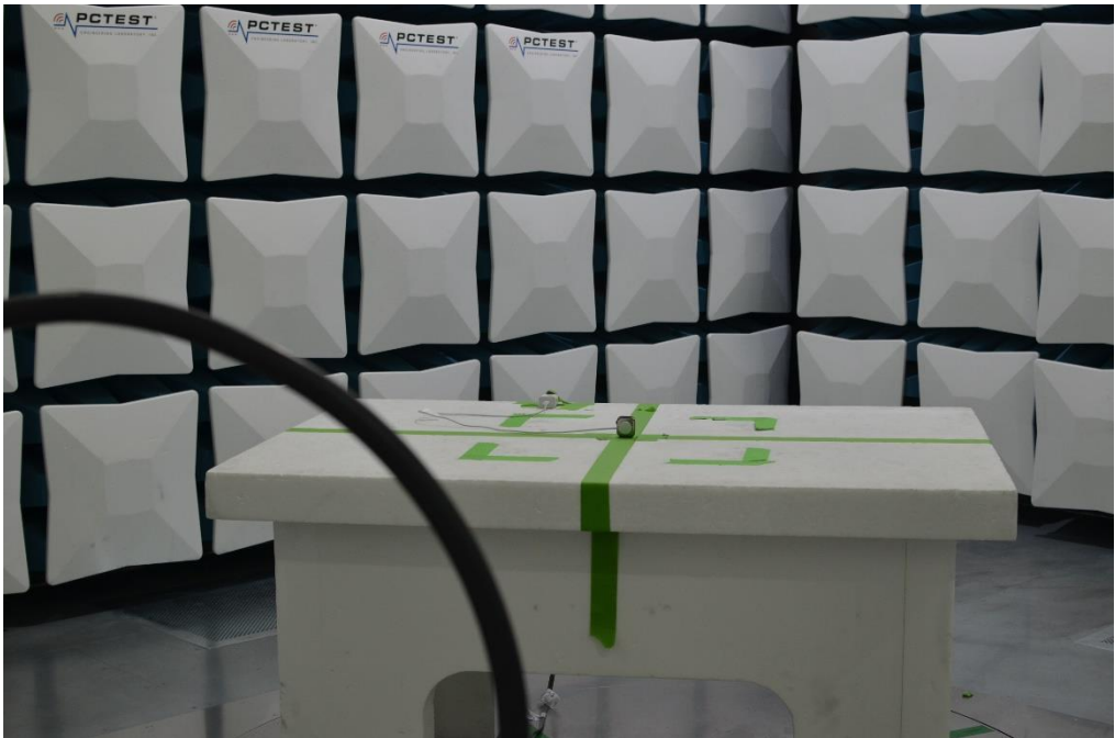
Figure 25: 9kHz-30MHz Test Setup (Front View)
