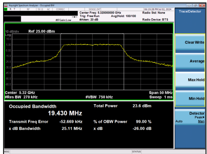
Plot 7-6. 26dB BW & 99% OBW (20MHz BW 802.11n – Ch. 64, MCS0)
