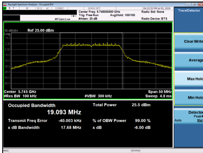
Plot 7-10. 6dB BW & 99% OBW (20MHz BW 802.11n – Ch. 149, MCS0)
