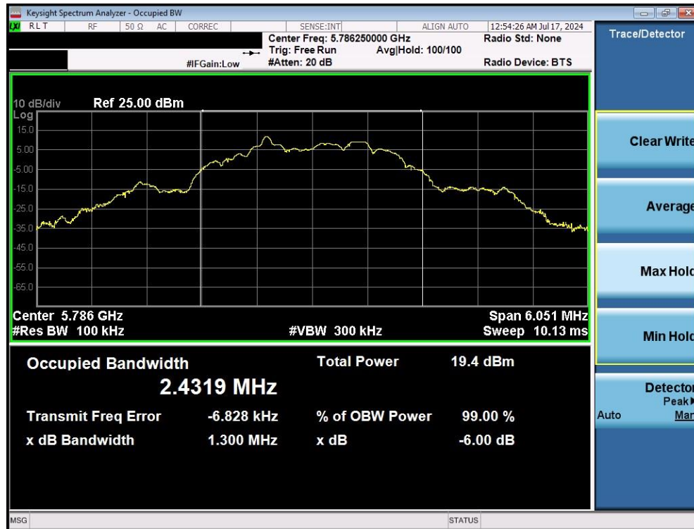
Plot 7-5. 6dB BW & 99% OBW (O-QPSK, 5786.25MHz, 500kpbs)
