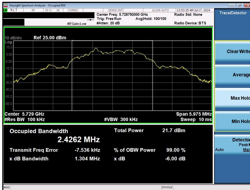
Plot 7-4. 6dB BW & 99% OBW (O-QPSK, 5728.75MHz, 500kpbs)
