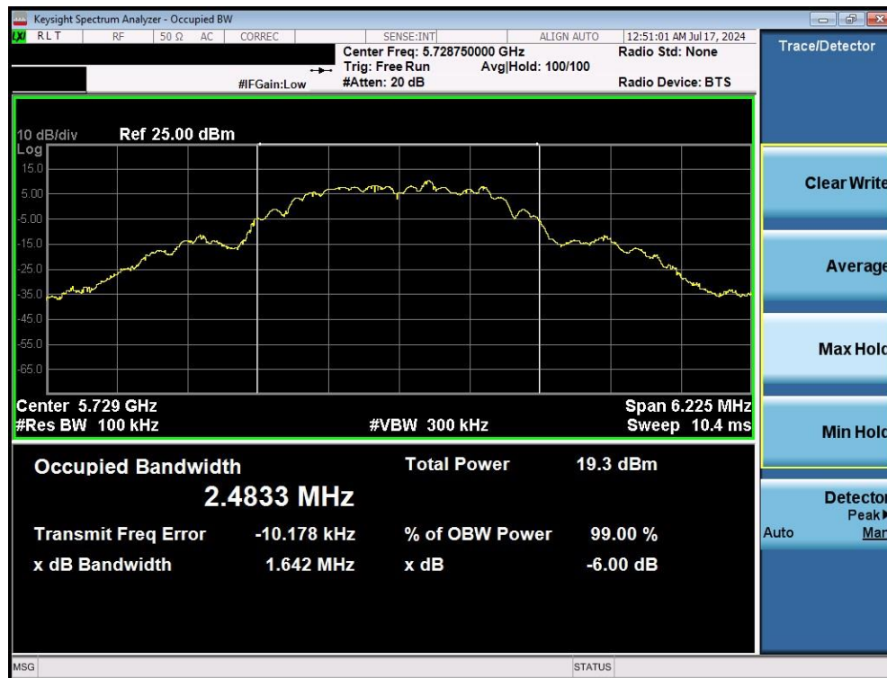
Plot 7-1. 6dB BW & 99% OBW (O-QPSK, 5728.75MHz, 250kbps)
