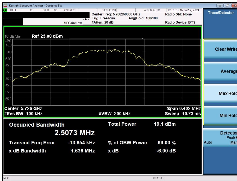
Plot 7-2. 6dB BW & 99% OBW (O-QPSK, 5786.25MHz, 250kbps)
