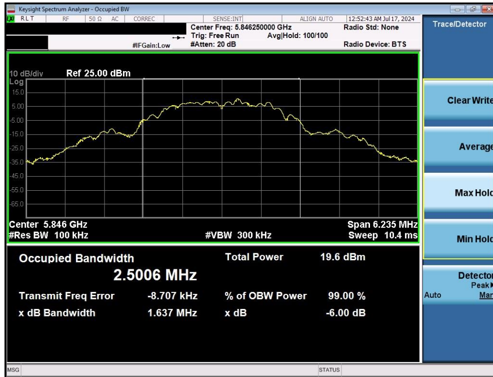
Plot 7-3. 6dB BW & 99% OBW (O-QPSK, 5846.25MHz, 250kpbs)
