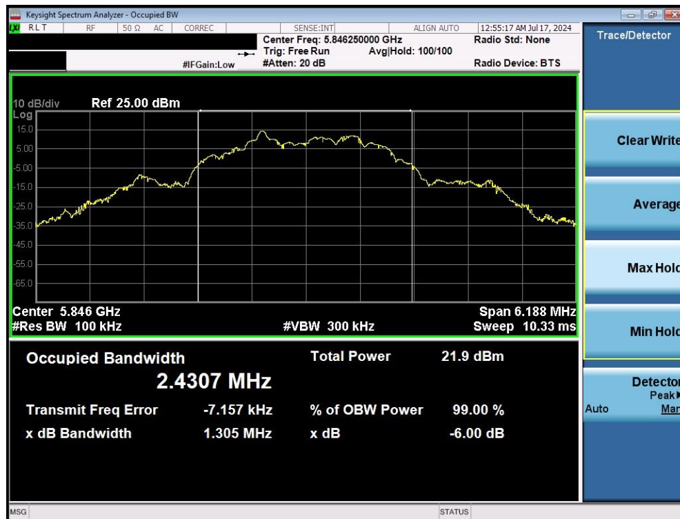
Plot 7-6. 6dB BW & 99% OBW (O-QPSK, 5846.25MHz, 500kpbs)
