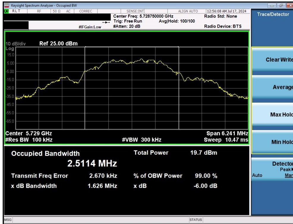
Plot 7-7. 6dB BW & 99% OBW (O-QPSK, 5728.75MHz, 1000kbps)
