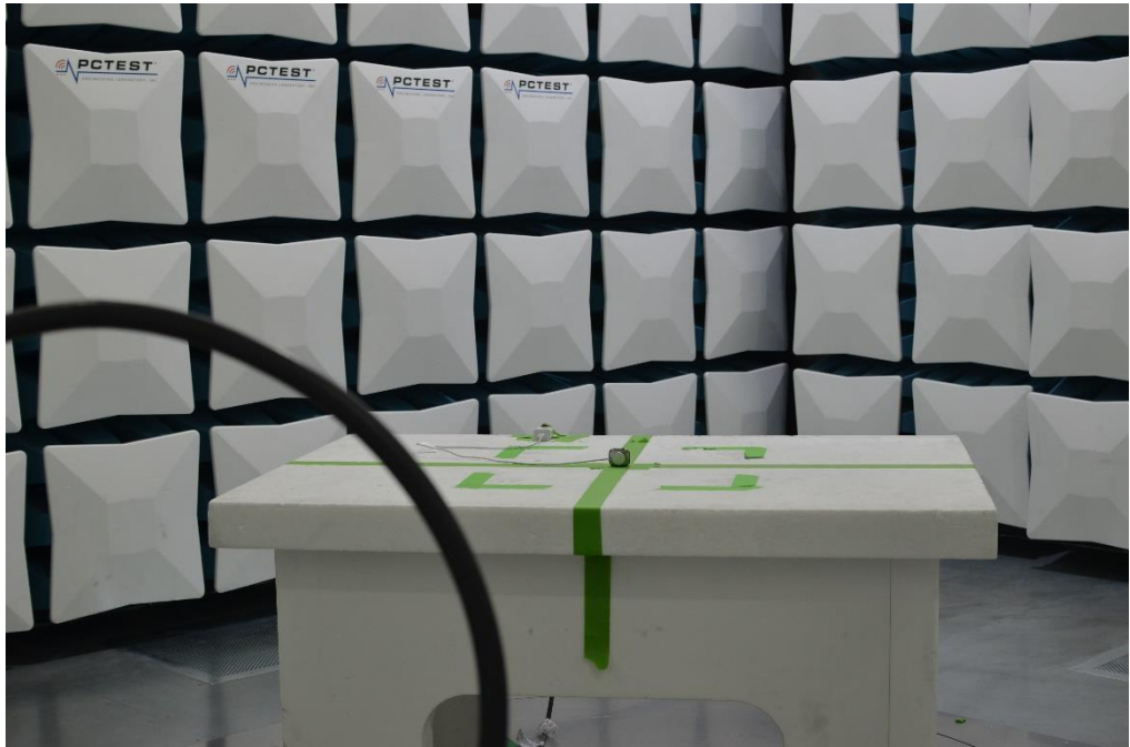
Figure 20: 9kHz-30MHz Test Setup (Front View)
