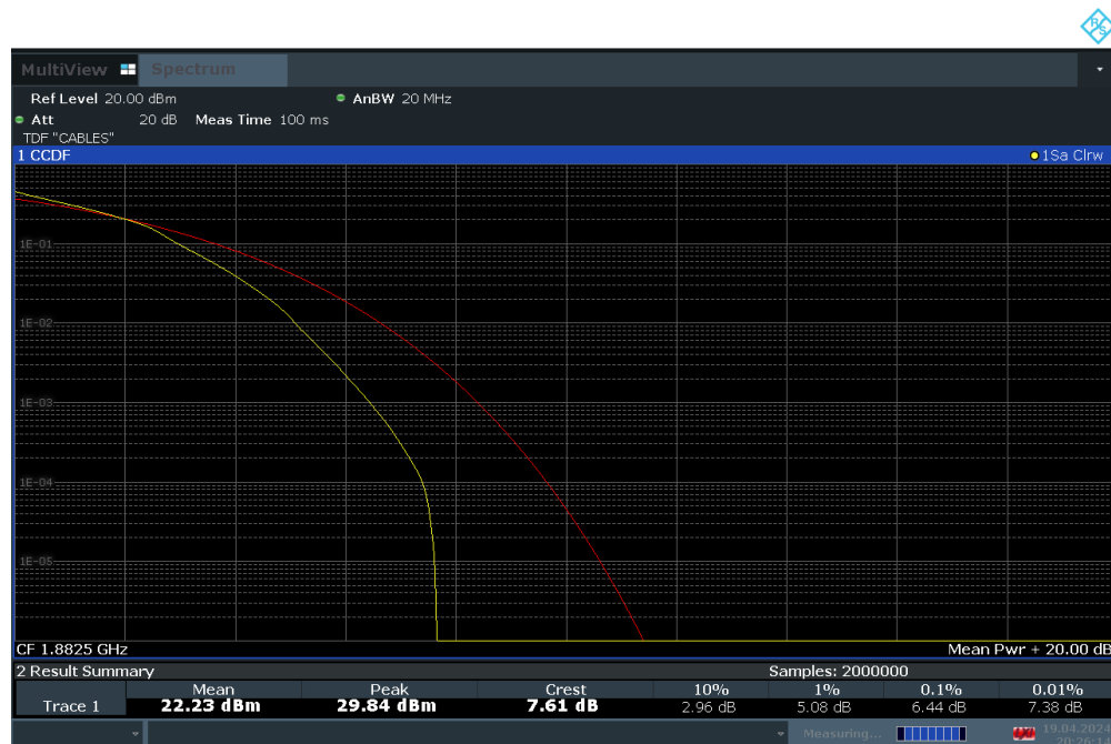
Plot 7-101. PAR Plot (LTE Band 25 - 20MHz 16-QAM - Full RB Configuration)
