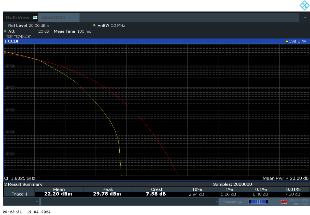
Plot 7-99. PAR Plot (LTE Band 25 - 15MHz 16-QAM - Full RB Configuration)
