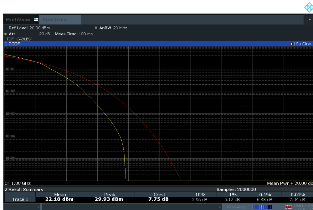
Plot 7-113. PAR Plot (LTE Band 2 - 20MHz 16-QAM - Full RB Configuration)
