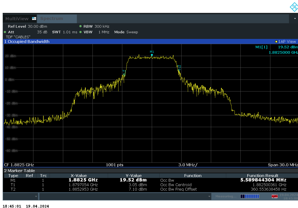
Plot 7-10. Occupied Bandwidth Plot (LTE Band 25/2 - 15MHz 16-QAM - Full RB Configuration)
