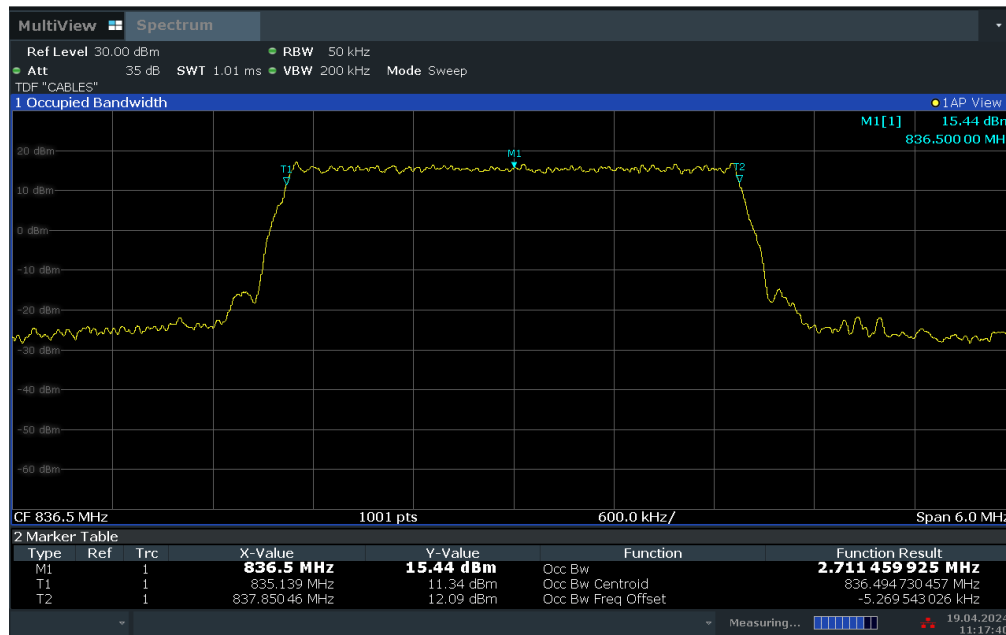
Plot 7-4. Occupied Bandwidth Plot (LTE Band 26/5 - 3MHz 16-QAM - Full RB Configuration)
