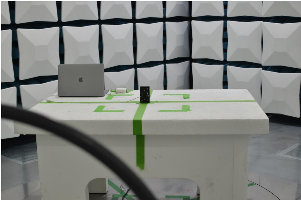
Figure 20: 9kHz-30MHz Test Setup (Front View)
