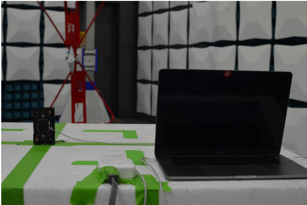
Figure 17: 30MHz-1GHz Test Setup (Rear View)
