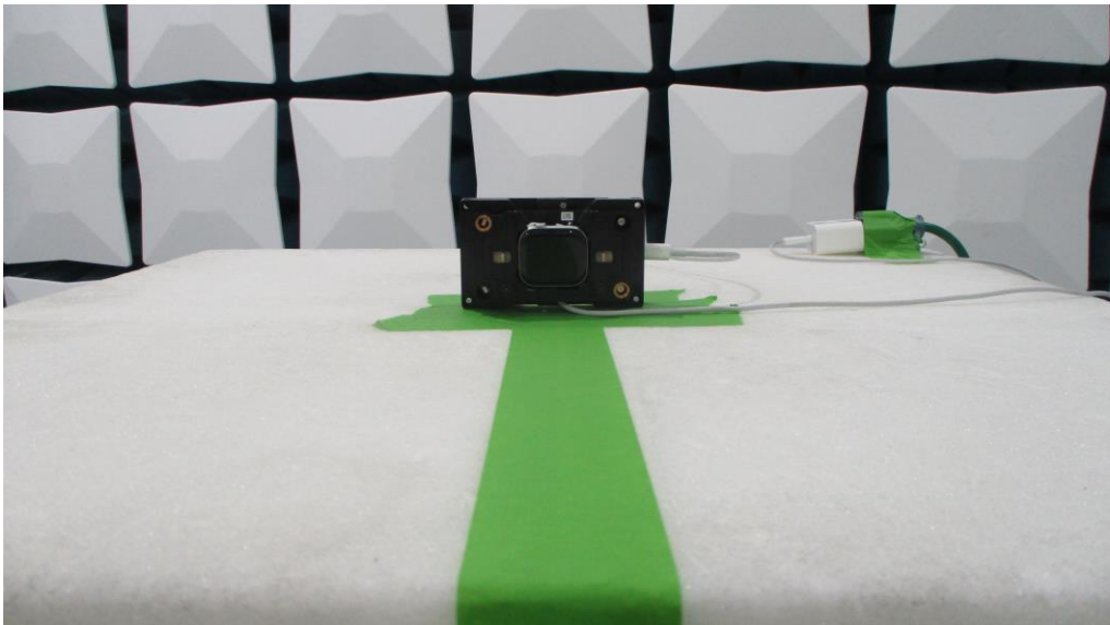
Figure 8: 1-18GHz Test Setup (Front View)
