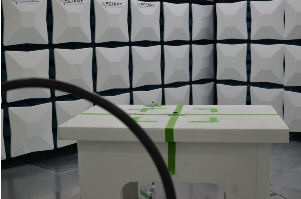
Figure 23: 9kHz-30MHz Test Setup (Front View)
