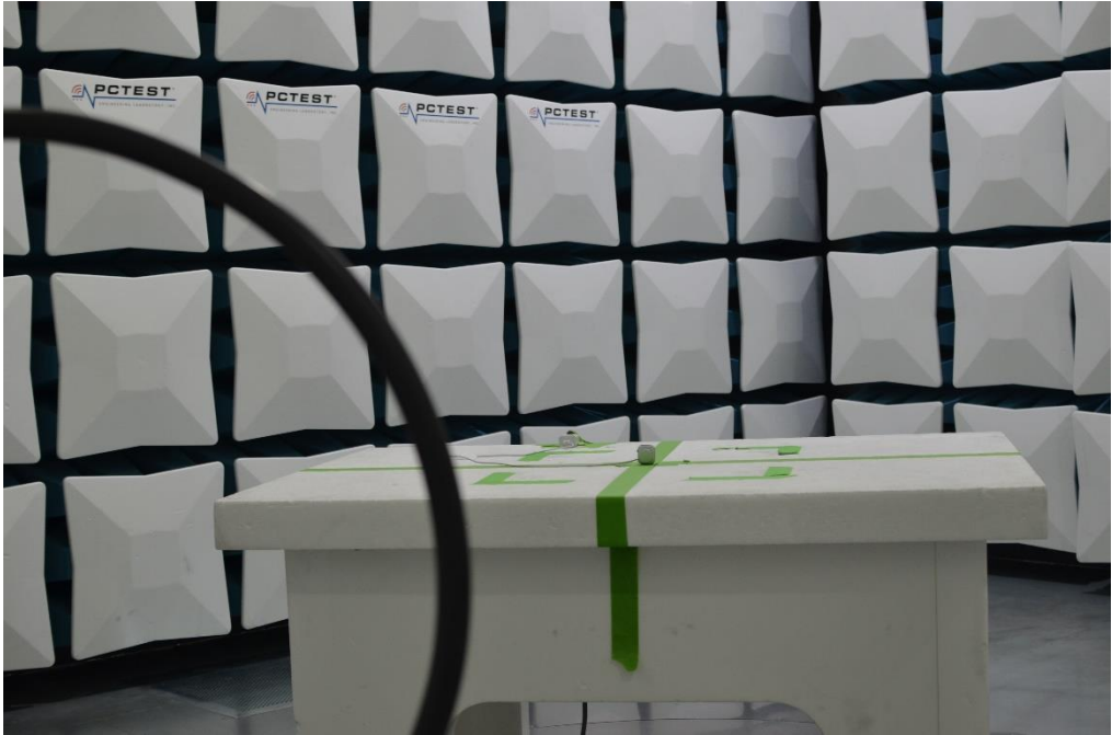
Figure 25: 9kHz-30MHz Test Setup (Front View)
