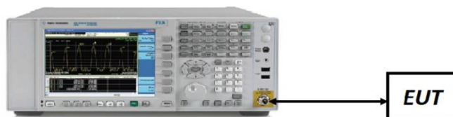
Figure 7-3. Test Instrument & Measurement Setup
