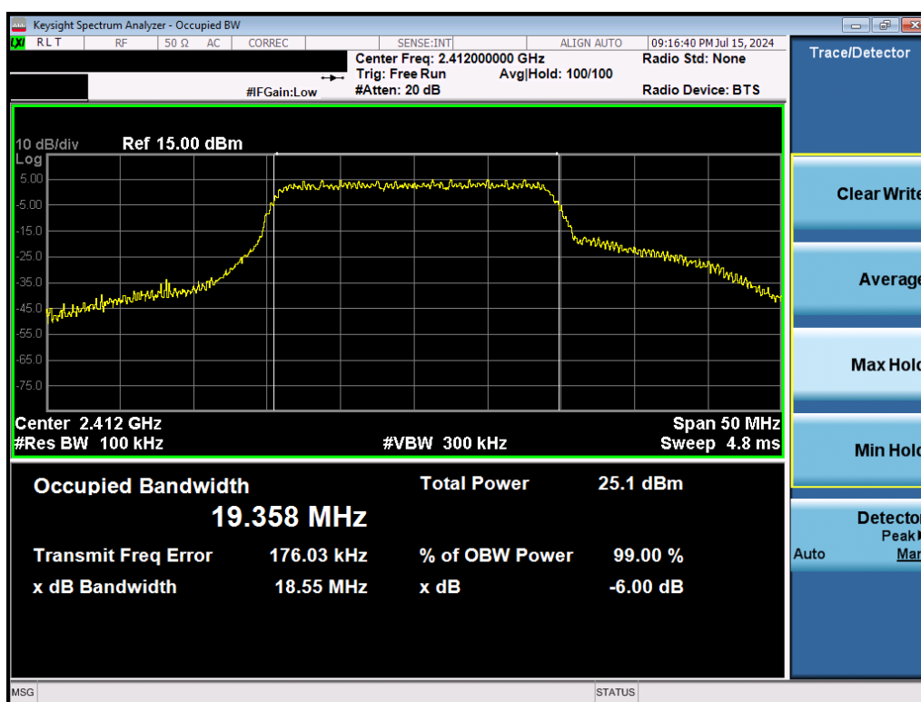
Plot 7-10. 6dB Bandwidth & 99% OBW Plot (802.11n (2.4GHz) – Ch. 1) – MCS7
