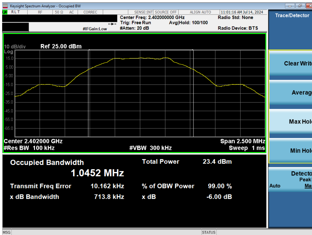
Plot 7-1. 6dB BW & 99% OBW Plot (Bluetooth (LE), 1Mbps, ePA – Ch. 0)
