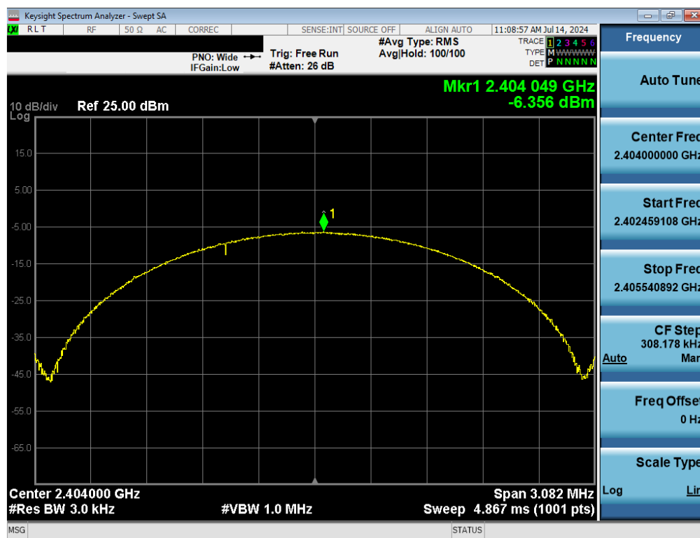
Plot 7-13. Power Spectral Density Plot (Bluetooth (LE), 2Mbps, ePA – Ch. 1)
