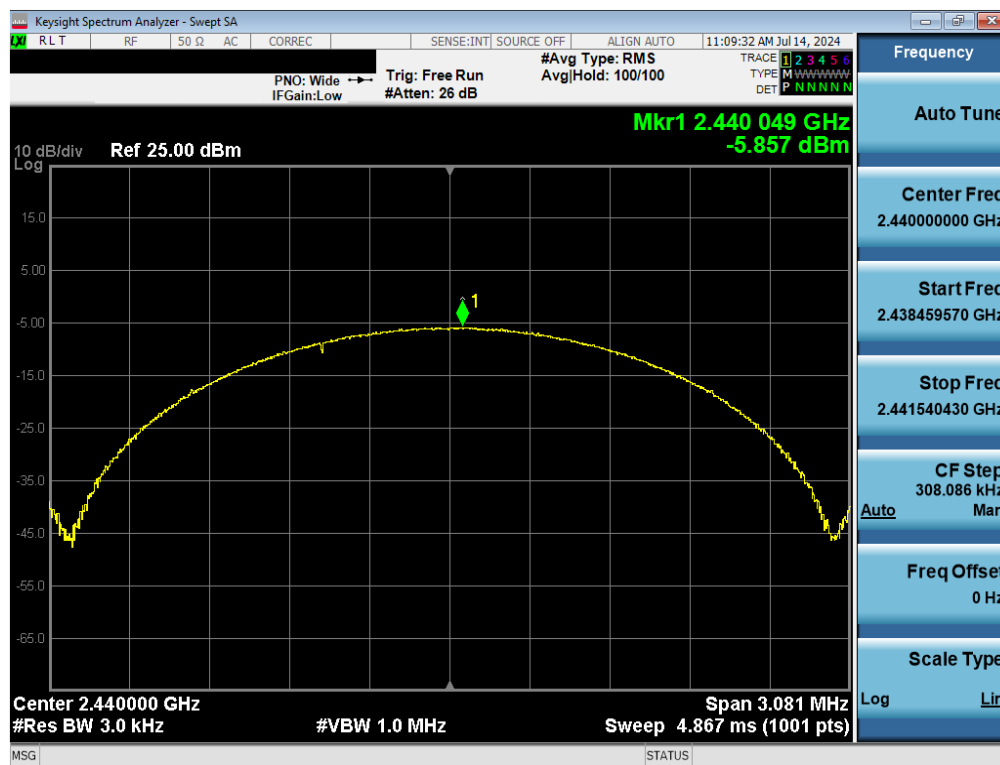
Plot 7-14. Power Spectral Density Plot (Bluetooth (LE), 2Mbps, ePA – Ch. 19)
