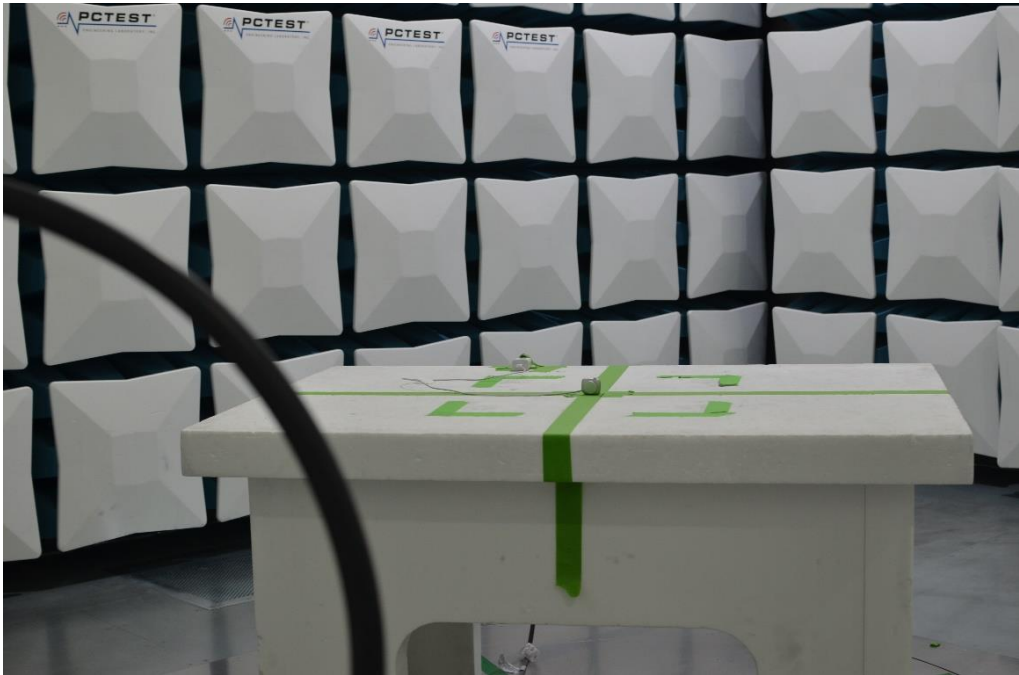
Figure 20: 9kHz-30MHz Test Setup (Front View)
