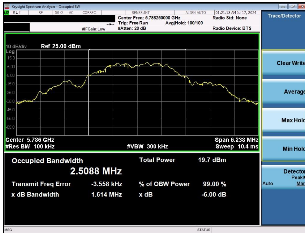
Plot 7-8. 6dB BW & 99% OBW (O-QPSK, 5786.25MHz, 1000kbps)
