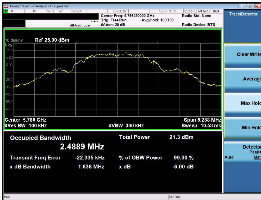
Plot 7-2. 6dB BW & 99% OBW (O-QPSK, 5786.25MHz, 250kpbs)
