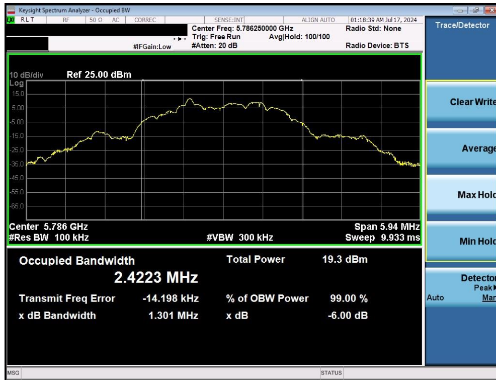
Plot 7-5. 6dB BW & 99% OBW (O-QPSK, 5786.25MHz, 500kpbs)
