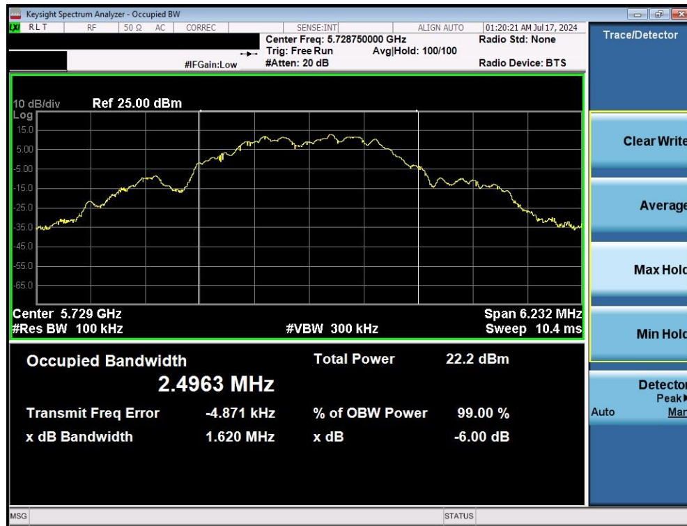
Plot 7-7. 6dB BW & 99% OBW (O-QPSK, 5728.75MHz, 1000kbps)
