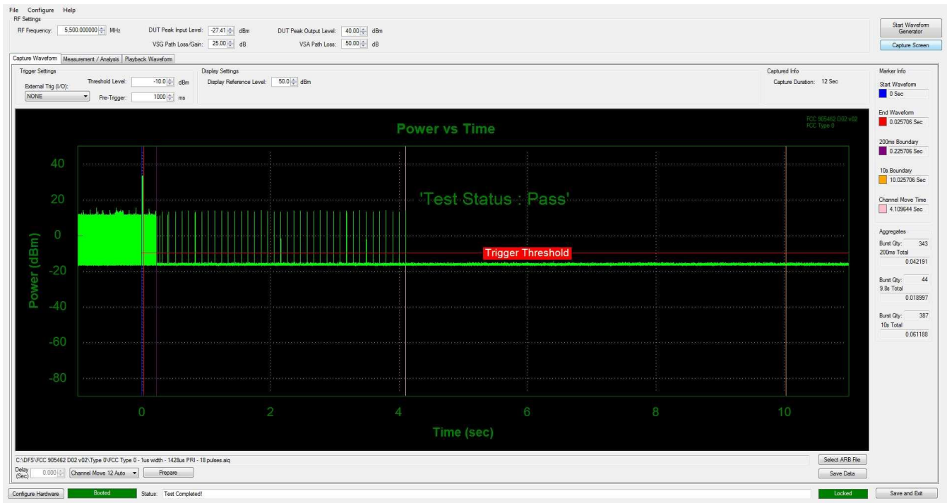
Figure 9-3. 5500MHz - Channel Move/ Closing Transmission Time - (20 MHz)
