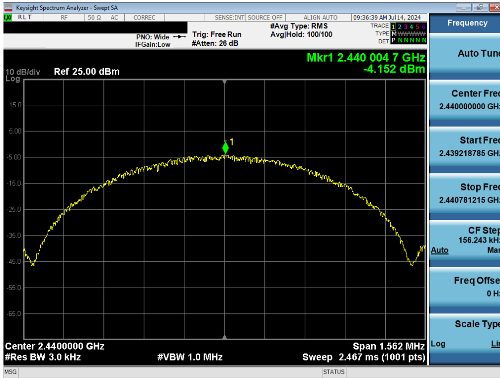
Plot 7-11. Power Spectral Density Plot (Bluetooth (LE), 1Mbps, iPA – Ch. 19)
