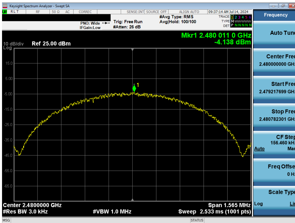
Plot 7-12. Power Spectral Density Plot (Bluetooth (LE), 1Mbps, iPA – Ch. 39)
