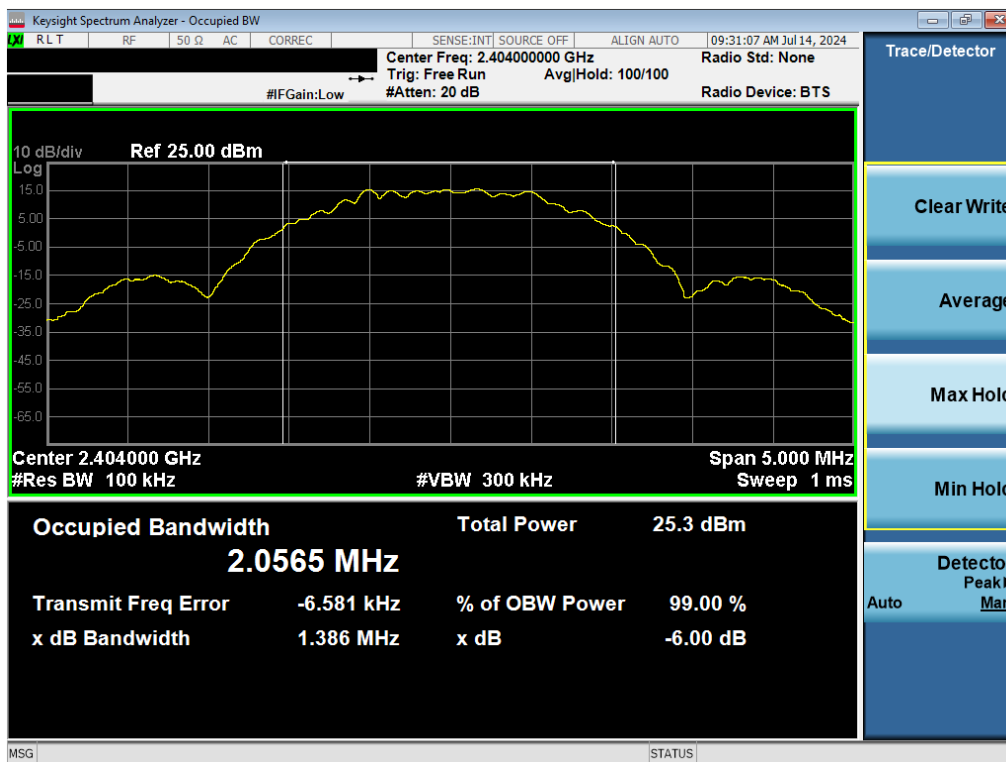
Plot 7-4. 6dB BW & 99% OBW Plot (Bluetooth (LE), 2Mbps, ePA – Ch. 1)
