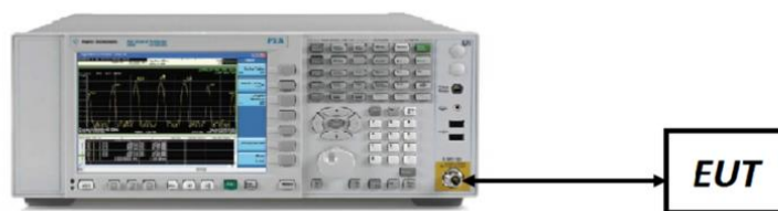
Figure 7-3. Test Instrument & Measurement Setup
