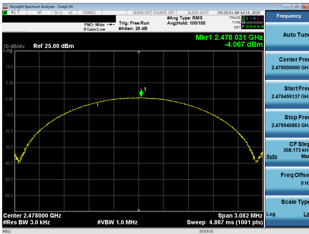
Plot 7-15. Power Spectral Density Plot (Bluetooth (LE), 2Mbps, ePA – Ch. 38)
