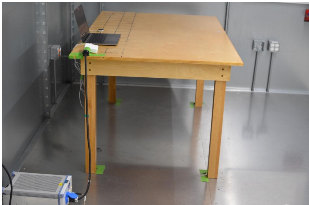
Figure 4: AC Line Conducted Emissions (Side View)
