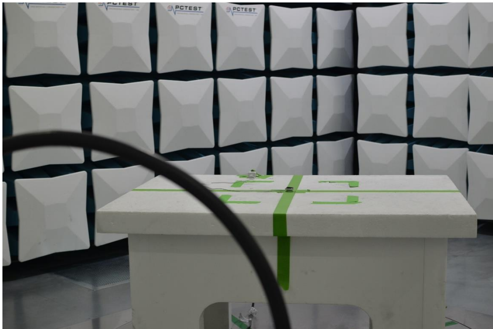
Figure 20: 9kHz-30MHz Test Setup (Front View)
