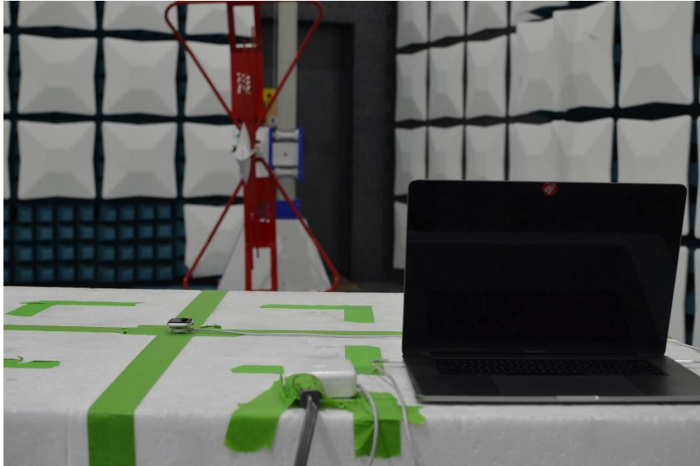
Figure 15: 30MHz-1GHz Test Setup (Rear View)
