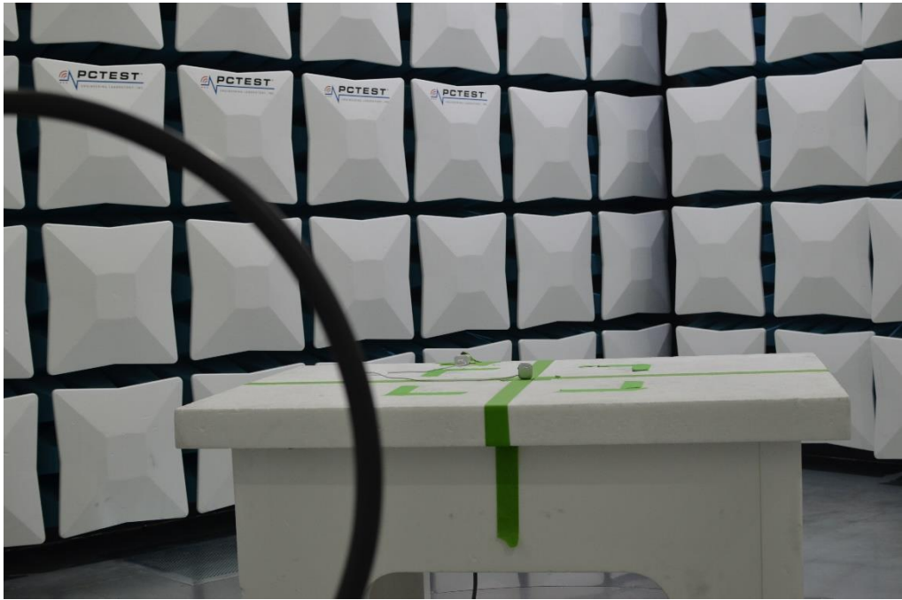
Figure 22: 9kHz-30MHz Test Setup (Front View)
