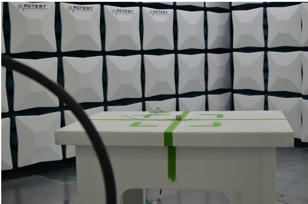
Figure 21: 9kHz-30MHz Test Setup (Front View)
