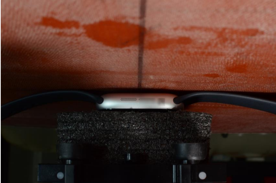
NFC SAR Test Setup Photo 7: Aluminum with Sport Wristband, Extremity, Back Side at 0.0 cm
