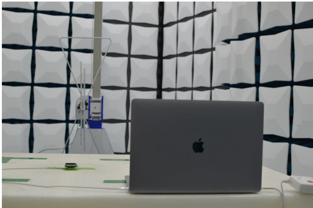
Figure 14: 30MHz-1GHz Test Setup (Rear View)
