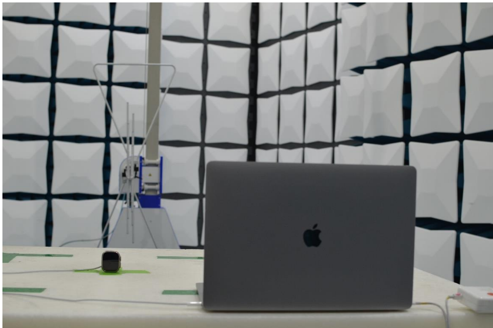
Figure 18: 30MHz-1GHz Test Setup (Rear View)
