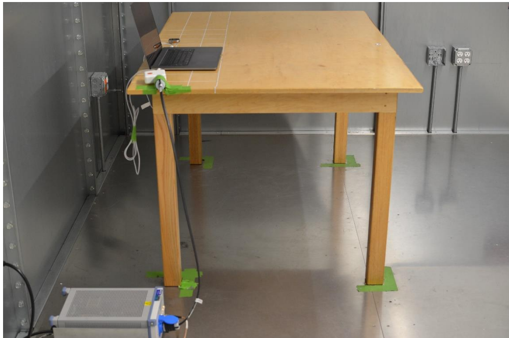
Figure 4: AC Line Conducted Emissions (Side View)
