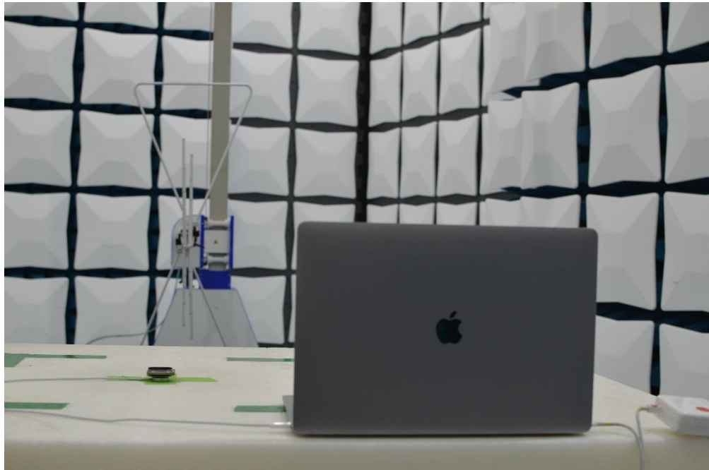
Figure 18: 30MHz-1GHz Test Setup (Rear View)
