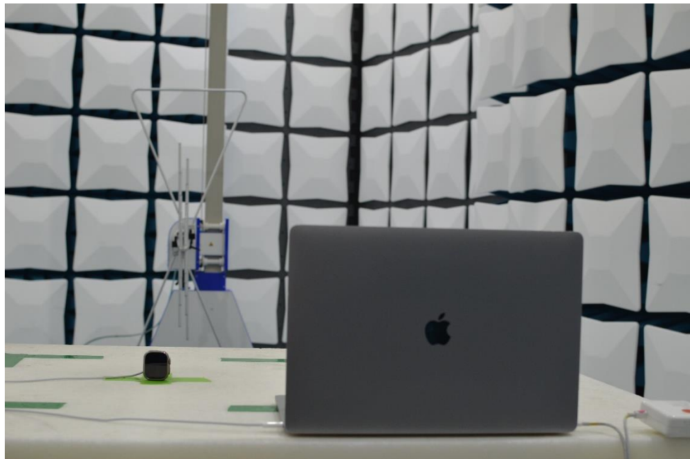
Figure 22: 30MHz-1GHz Test Setup (Rear View)
