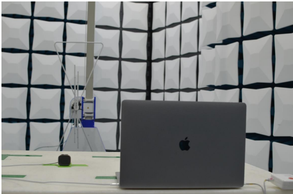
Figure 20: 30MHz-1GHz Test Setup (Rear View)
