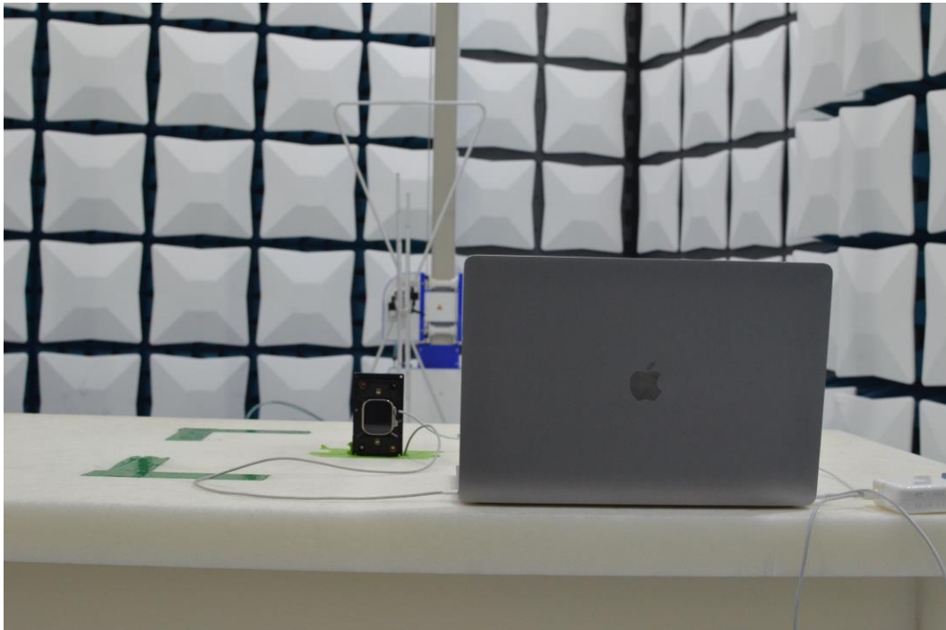
Figure 17: 30MHz-1GHz Test Setup (Rear View)
