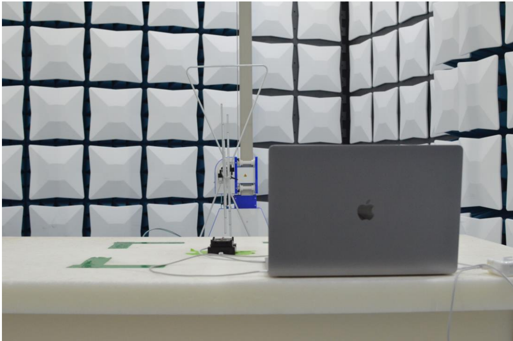
Figure 13: 30MHz-1GHz Test Setup (Rear View)
