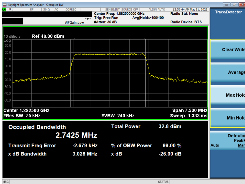
Plot 7-4. Occupied Bandwidth Plot (LTE Band 25/2 - 3MHz 16-QAM - Full RB Configuration)
