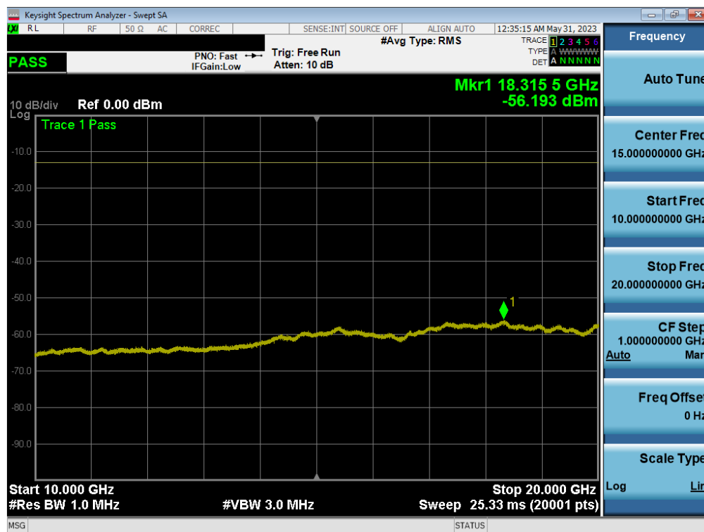
Plot 7-22. Conducted Spurious Plot (LTE Band 25/2 - 20MHz QPSK - RB Size 1, RB Offset 0 - High Channel)
