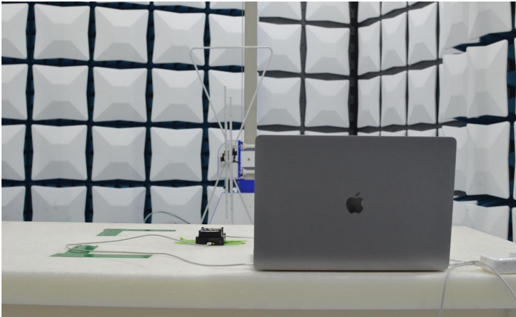
Figure 13: 30MHz-1GHz Test Setup (Rear View)
