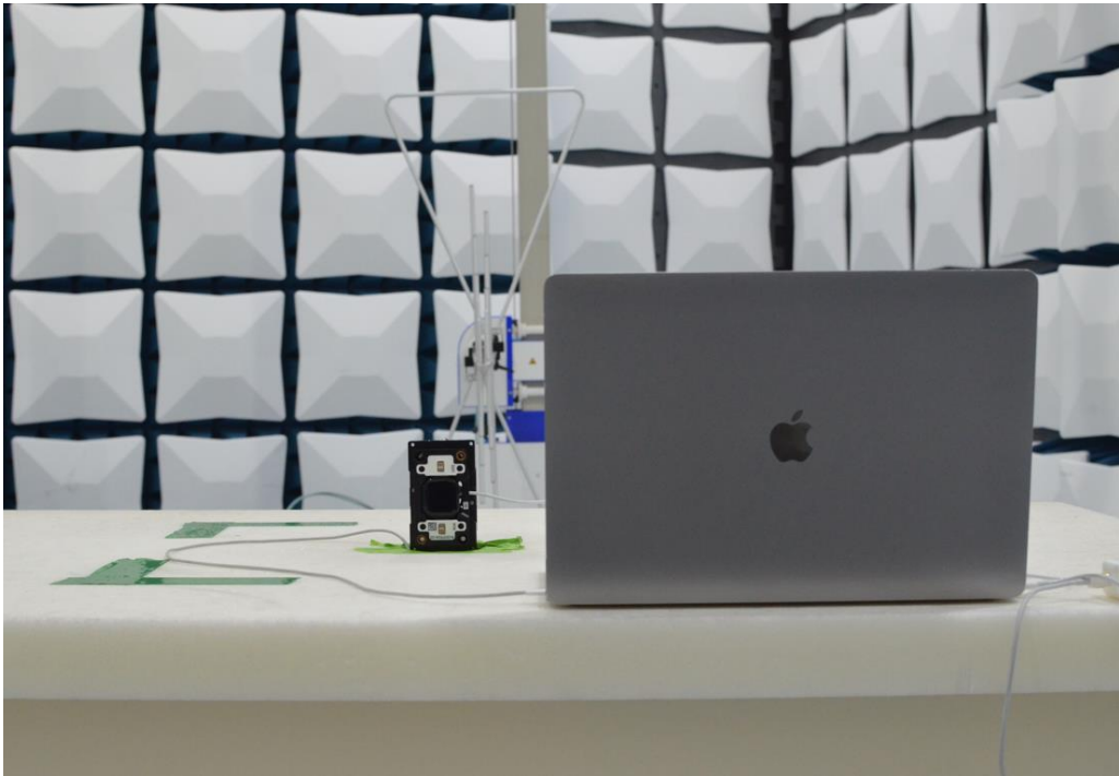
Figure 17: 30MHz-1GHz Test Setup (Rear View)
