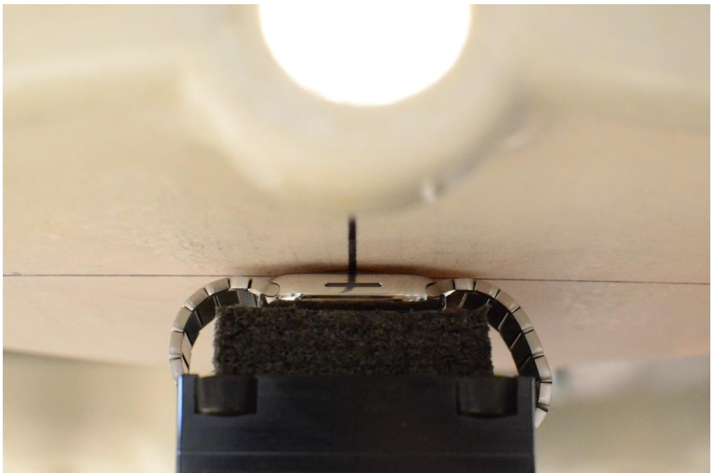
SAR Test Setup Photo 11: Stainless Steel with Metal Links Wristband, Extremity, Back Side at 0mm
