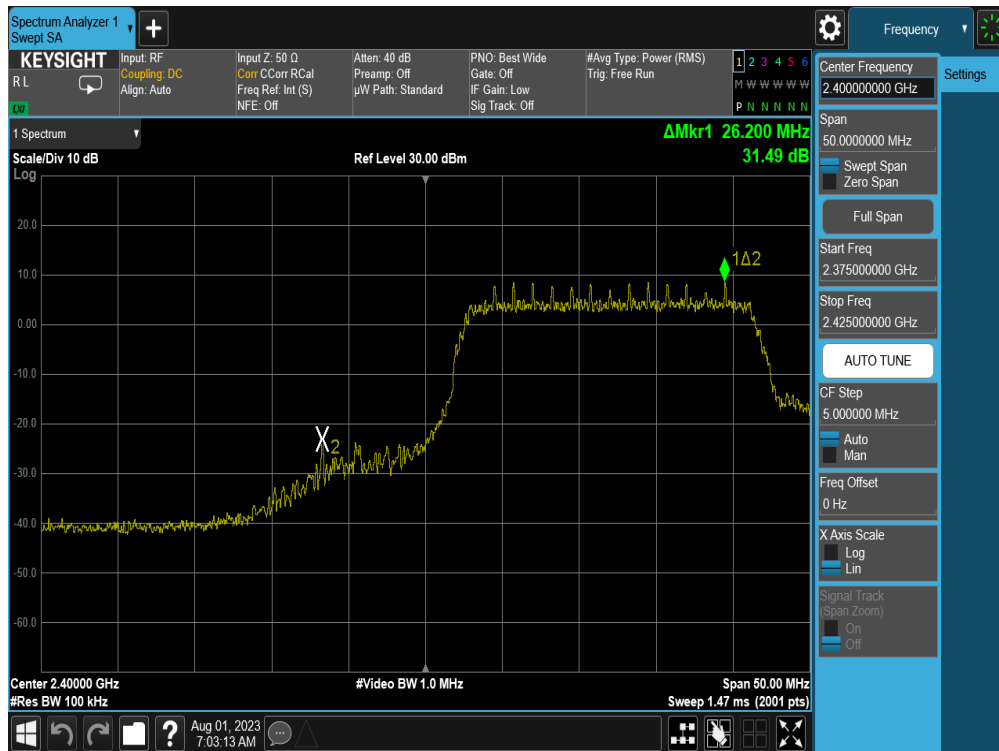
Plot 7-36. Band Edge Plot (802.11n (2.4GHz) – Ch. 1) – MCS0
