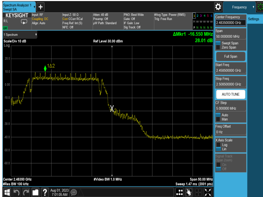
Plot 7-35. Band Edge Plot (802.11g – Ch. 13) – 6Mbps
