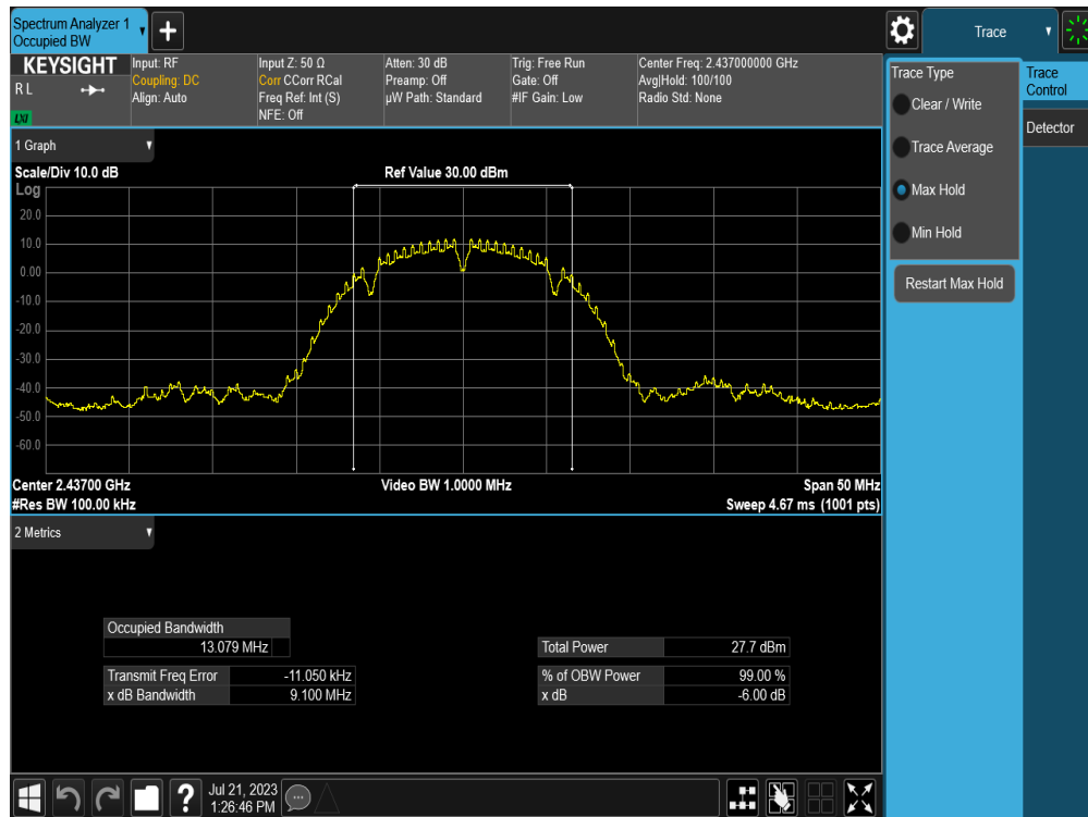
Plot 7-2. 6dB Bandwidth & 99% OBW Plot (802.11b – Ch. 6) – 1Mbps
