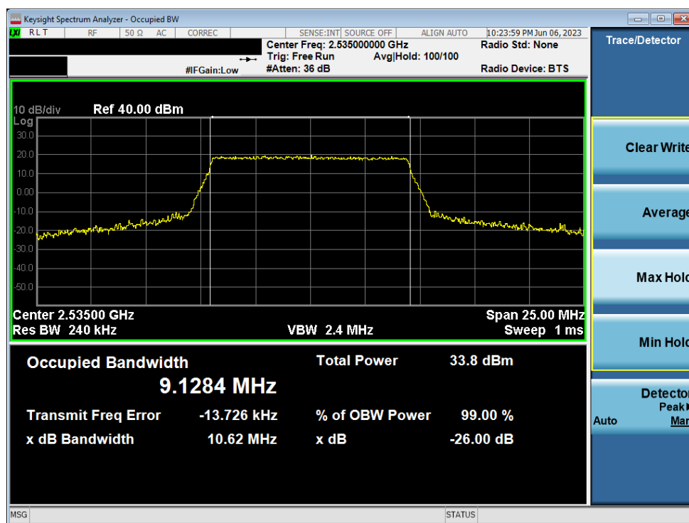
Plot 7-3. Occupied Bandwidth Plot (LTE Band 7 - 10MHz QPSK - Full RB)
