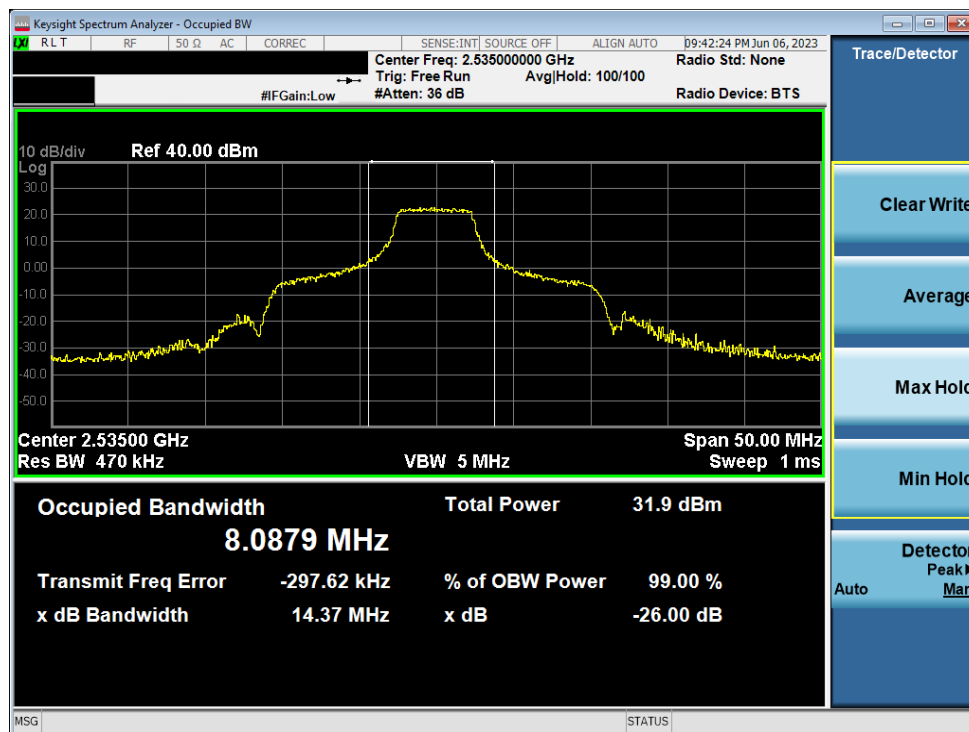
Plot 7-8. Occupied Bandwidth Plot (LTE Band 7 - 20MHz 16-QAM - Full RB)
