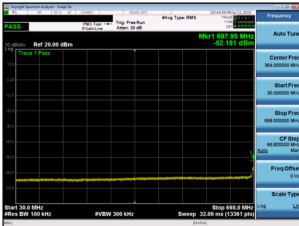
Plot 7-38. Conducted Spurious Plot (LTE Band 12/17 - 10MHz QPSK - RB Size 1, RB Offset 0 - Mid Channel)
