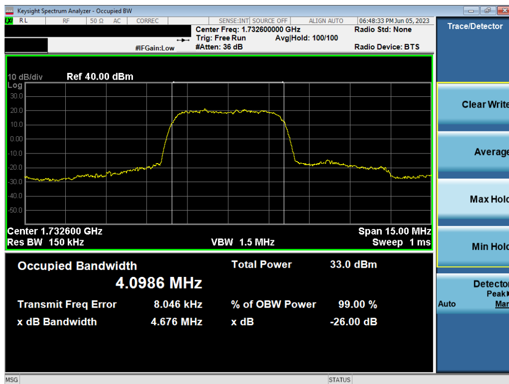
Plot 7-25. Occupied Bandwidth Plot (WCDMA, Ch. 1413)
