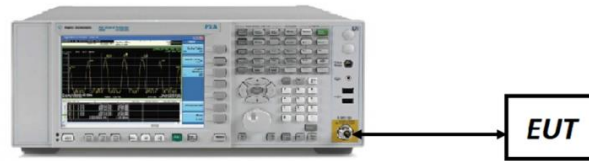
Figure 7-1. Test Instrument & Measurement Setup
