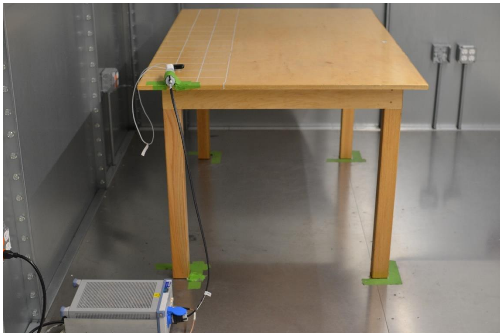
Figure 2: AC Line Conducted Emissions (Side View)
