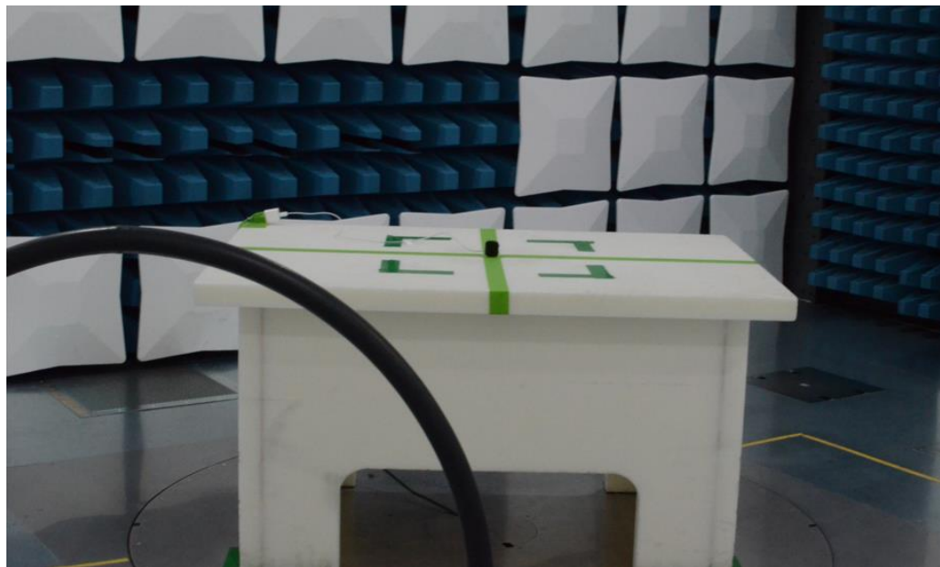
Figure 22: 9kHz-30MHz Test Setup (Front View)
