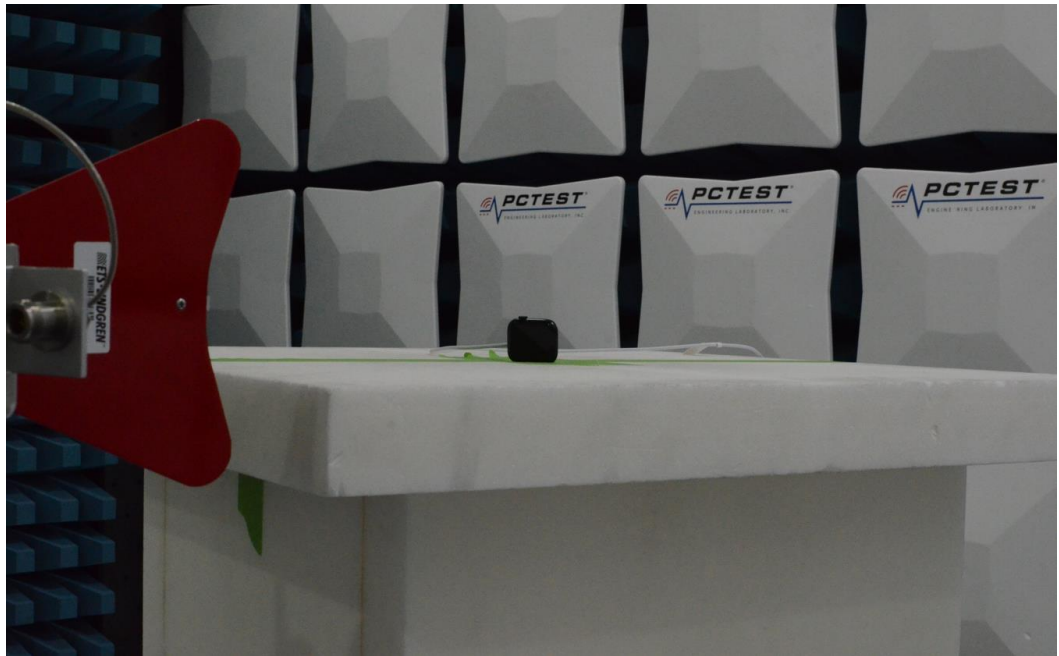
Figure 6: Above 960MHz Test Setup
