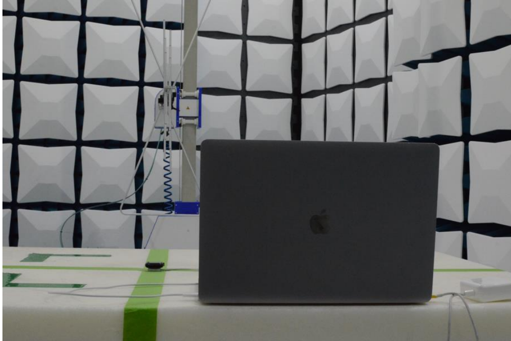
Figure 15: 30MHz-1GHz Test Setup (Rear View)
