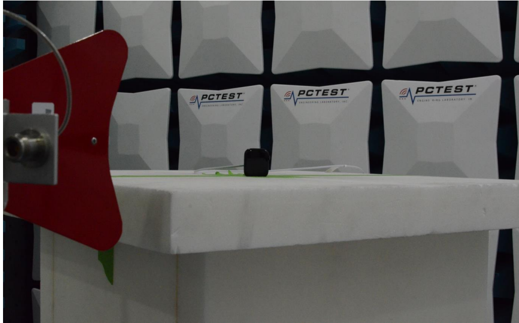
Figure 7: Above 960MHz Test Setup
