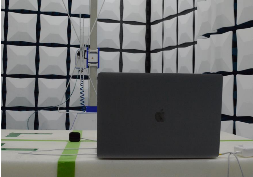
Figure 17: 30MHz-1GHz Test Setup (Rear View)
