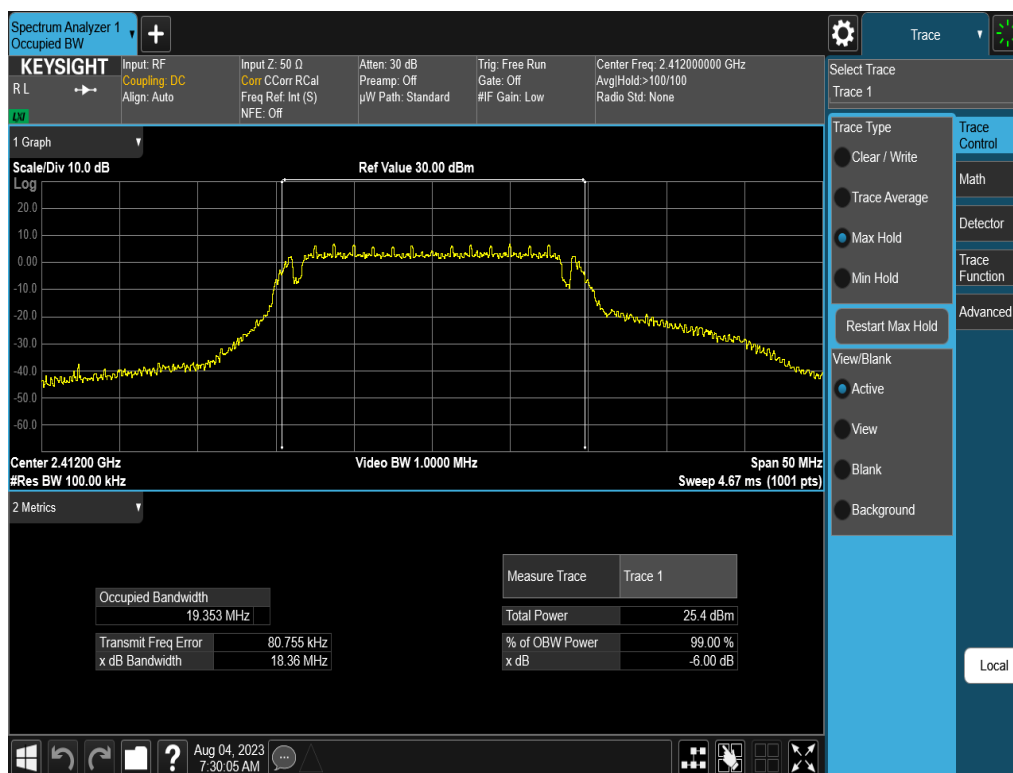
Plot 7-4. 6dB Bandwidth & 99% OBW Plot (802.11g – Ch. 1) – 6Mbps
