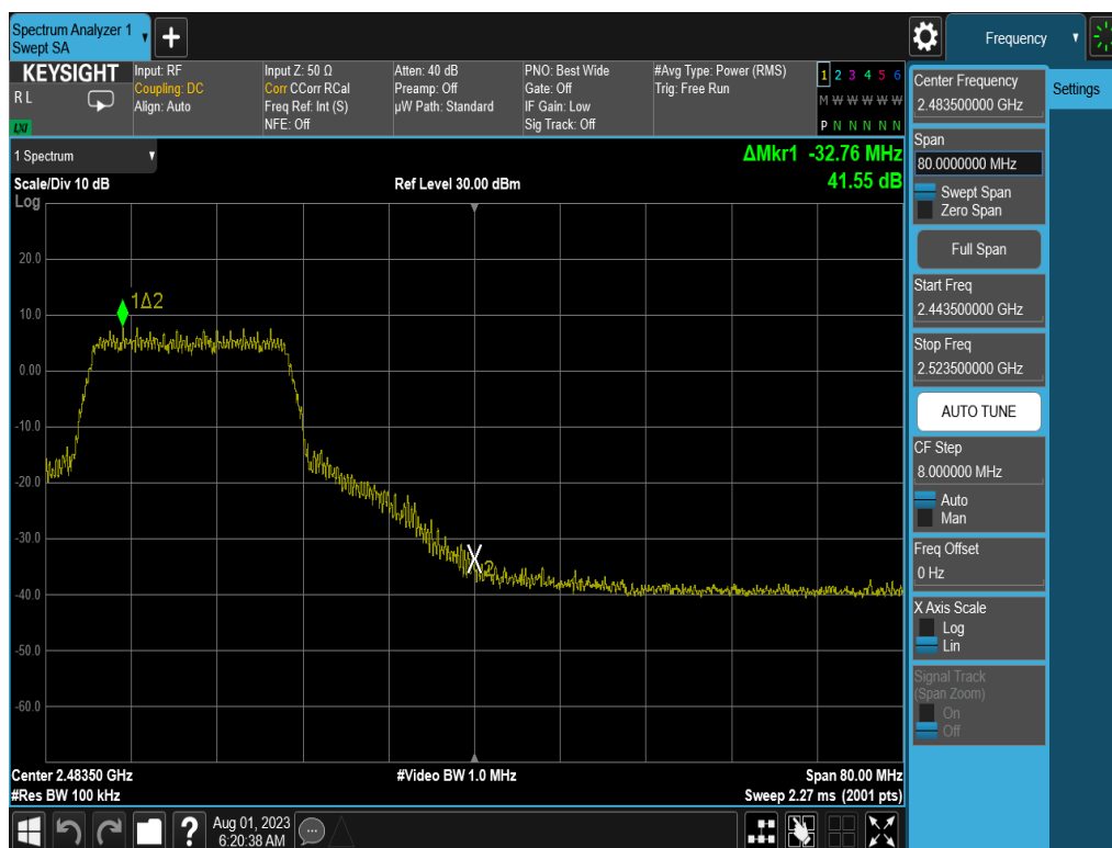
Plot 7-42. Band Edge Plot (802.11n (2.4GHz) – Ch. 10) – MCS7
