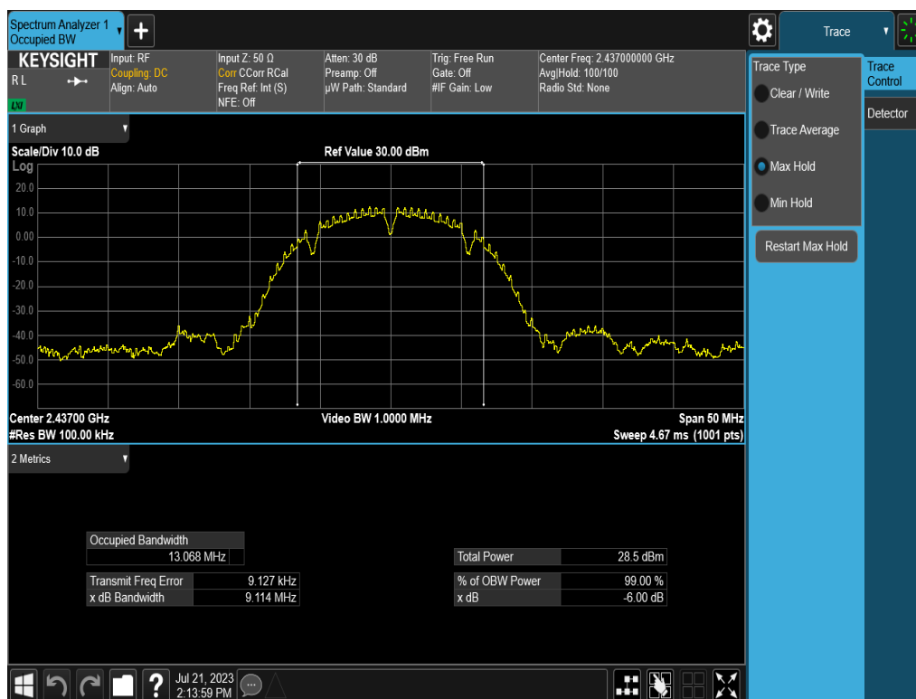
Plot 7-2. 6dB Bandwidth & 99% OBW Plot (802.11b – Ch. 6) – 1Mbps
