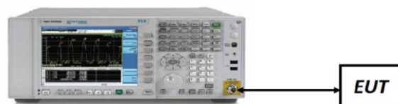
Figure 7-4. Test Instrument & Measurement Setup
