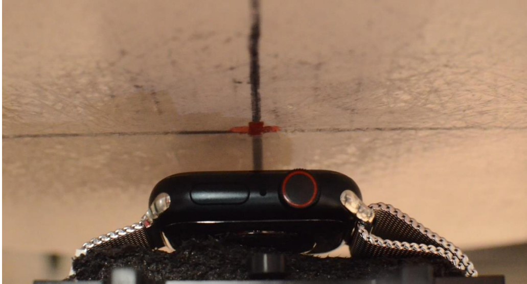
SAR Test Setup Photo 3: Aluminum with Metal Loop Wristband, Head, Front Side at 1.0 cm
