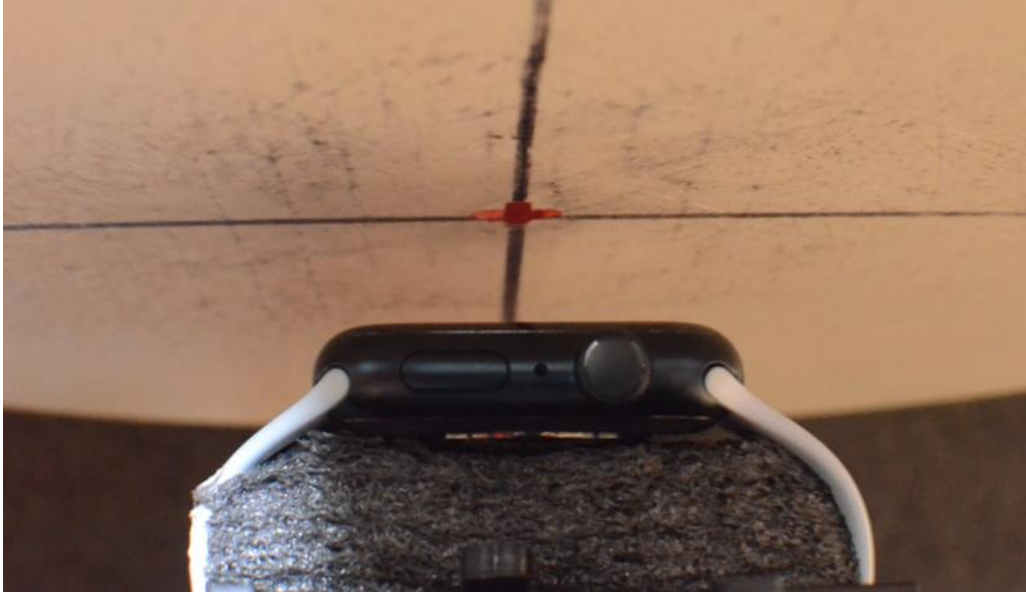
SAR Test Setup Photo 1: Aluminum with Sport Wristband, Head, Front Side at 1.0 cm
