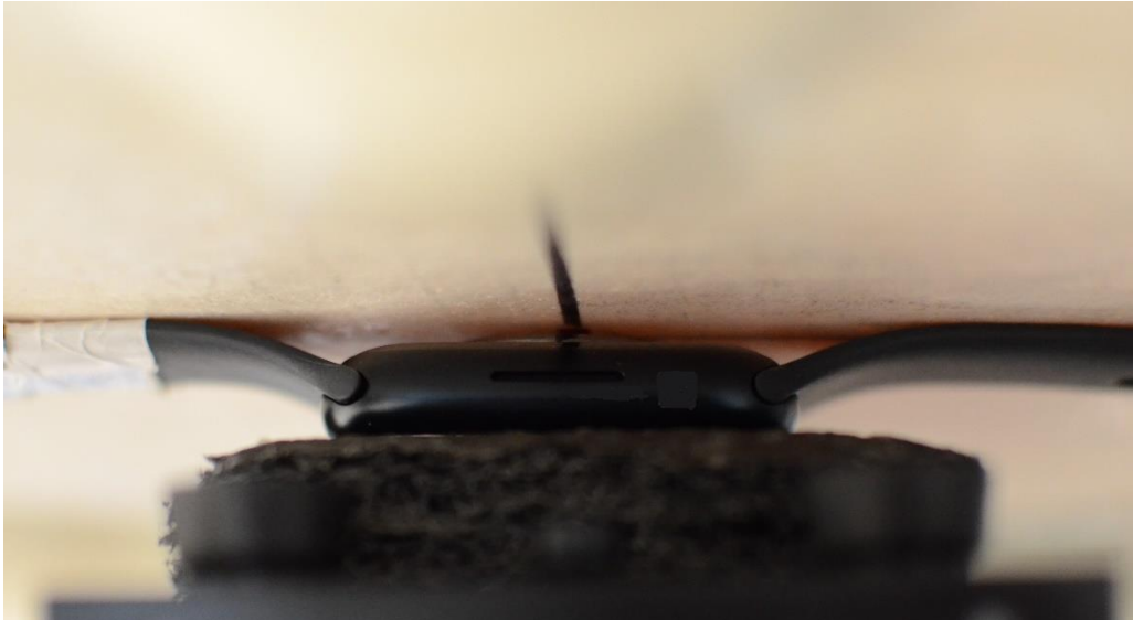
SAR Test Setup Photo 4: Aluminum with Sports Wristband, Extremity, Back Side at 0.0 cm
