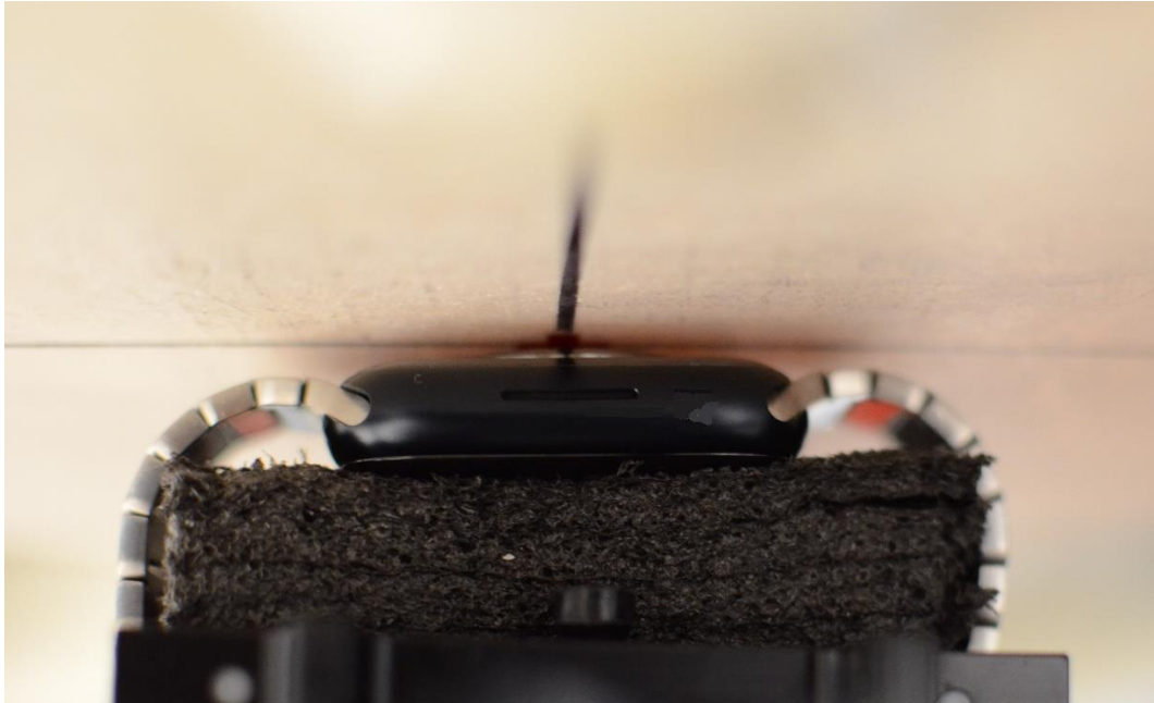
SAR Test Setup Photo 5: Aluminum with Metal Links Wristband, Extremity, Back Side at 0.0 cm
