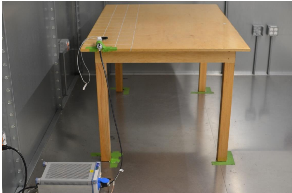
Figure 2: AC Line Conducted Emissions (Side View)
