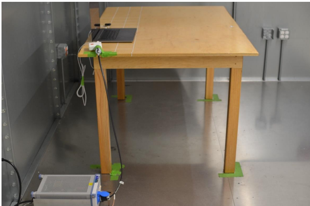
Figure 4: AC Line Conducted Emissions (Side View)
