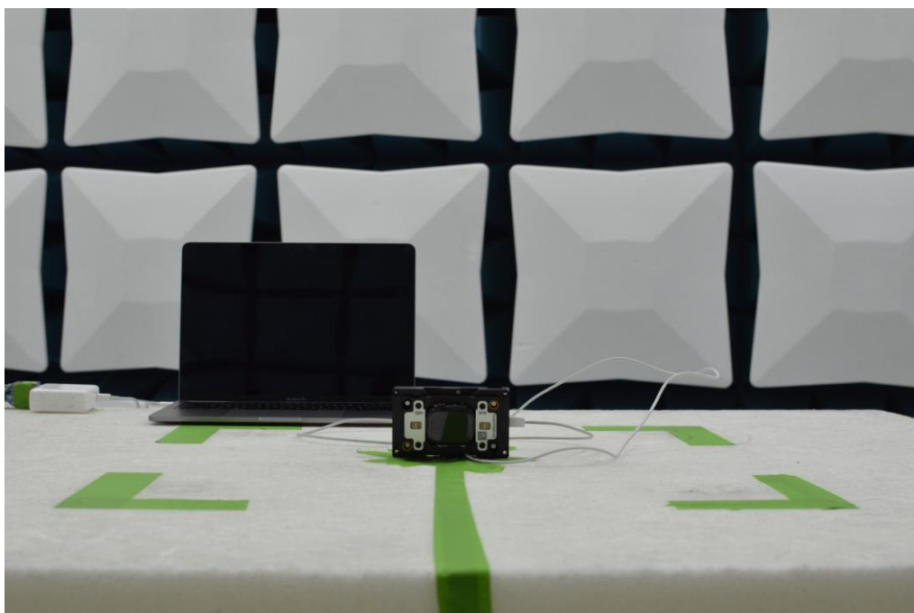
Figure 14: 30MHz-1GHz Test Setup (Front View)
