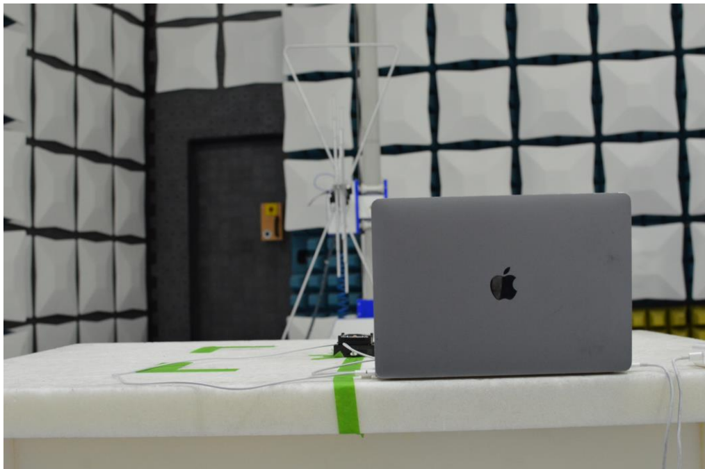
Figure 13: 30MHz-1GHz Test Setup (Rear View)
