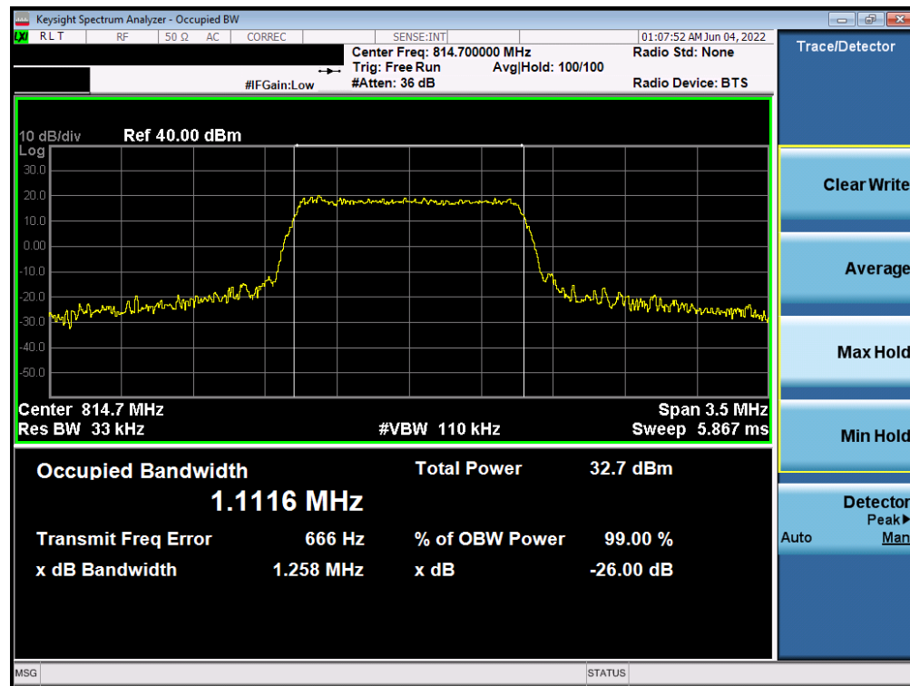
Plot 7-2. Occupied Bandwidth Plot (LTE Band 26 - 1.4MHz 16-QAM - Full RB Configuration)
