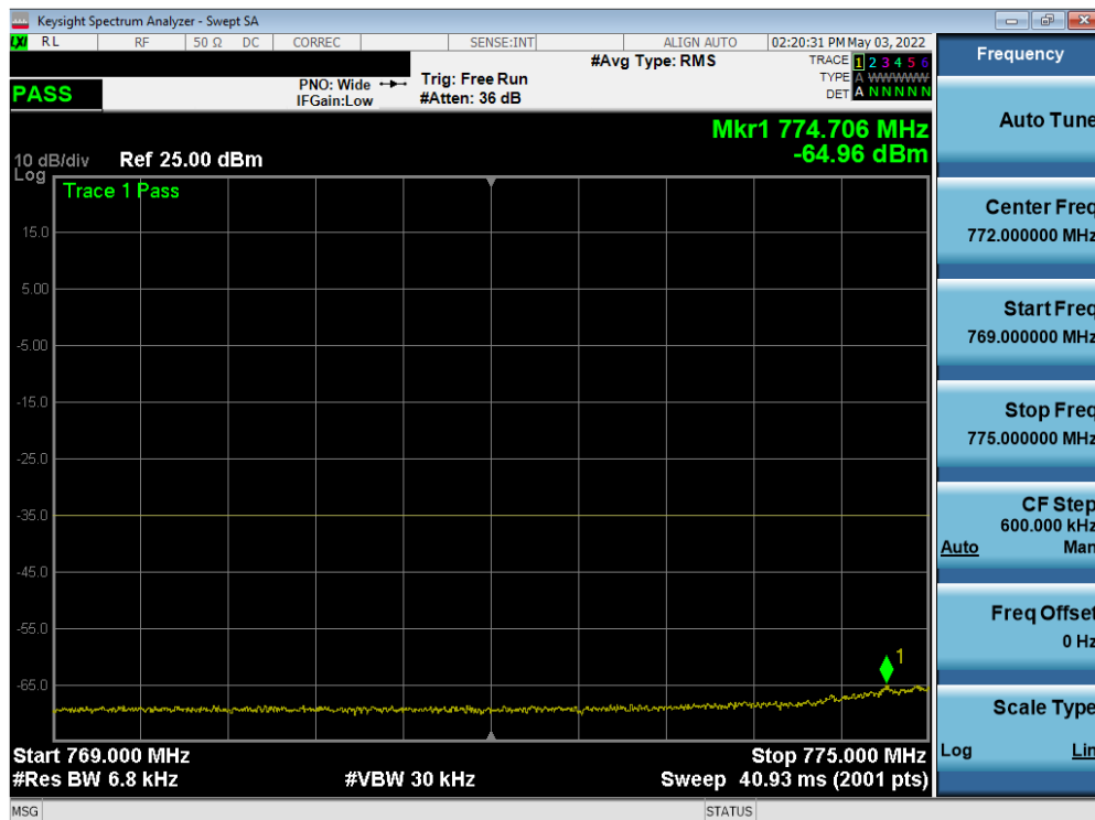
Plot 7-43. Lower Emission Mask Plot (LTE Band 14, 10MHz QPSK - RB Size 50)
