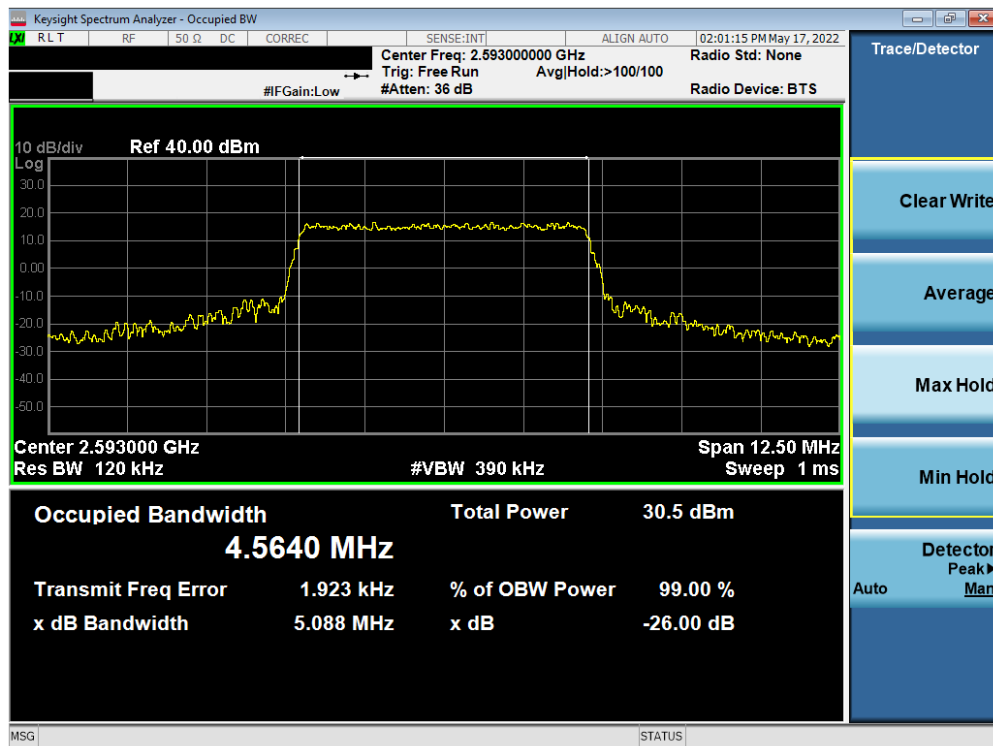
Plot 7-9. Occupied Bandwidth Plot (LTE Band 41 - 5MHz QPSK - Full RB)
