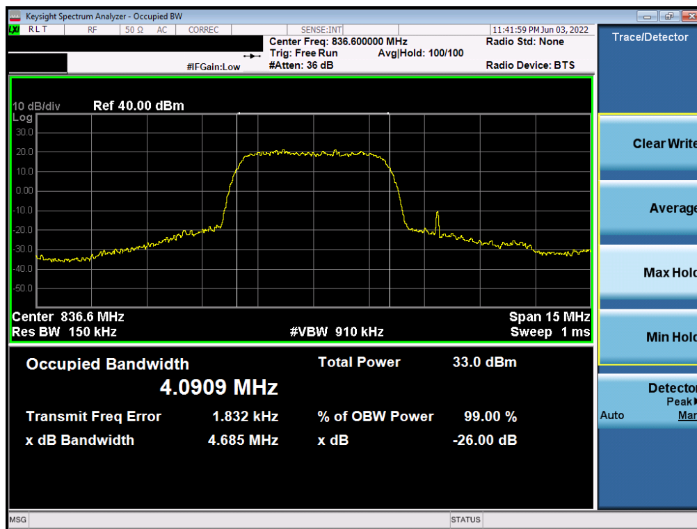
Plot 7-9. Occupied Bandwidth Plot (WCDMA, Ch. 4183)
