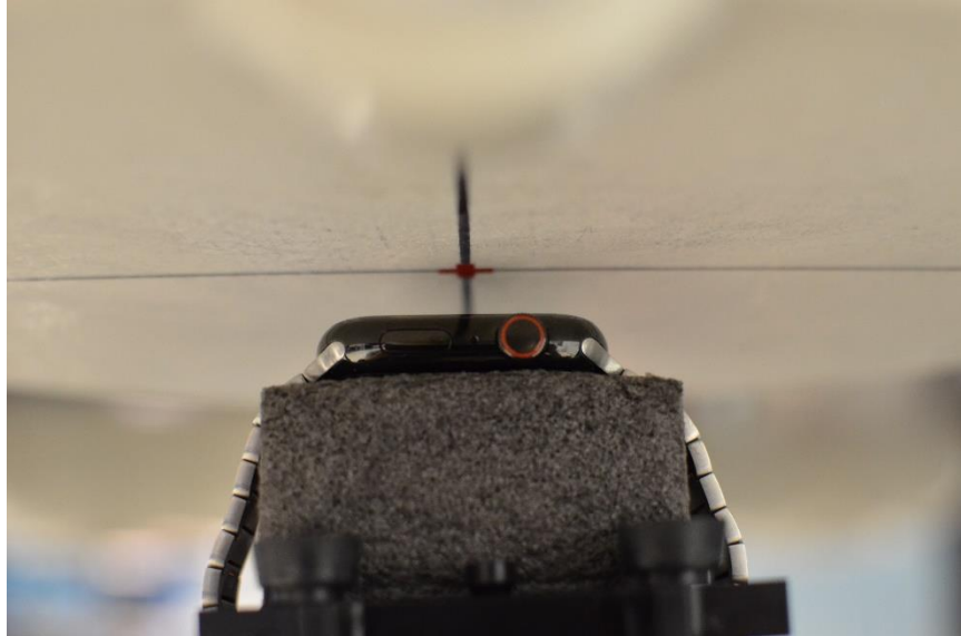
SAR Test Setup Photo 5: Stainless Steel with Metal Links Wristband, Head, Front Side at 1.0 cm
