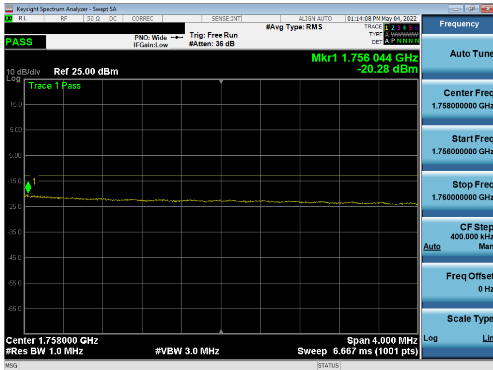
Plot 7-103. Upper Extended Band Edge Plot (LTE Band 4 - 20MHz QPSK – Full RB)
