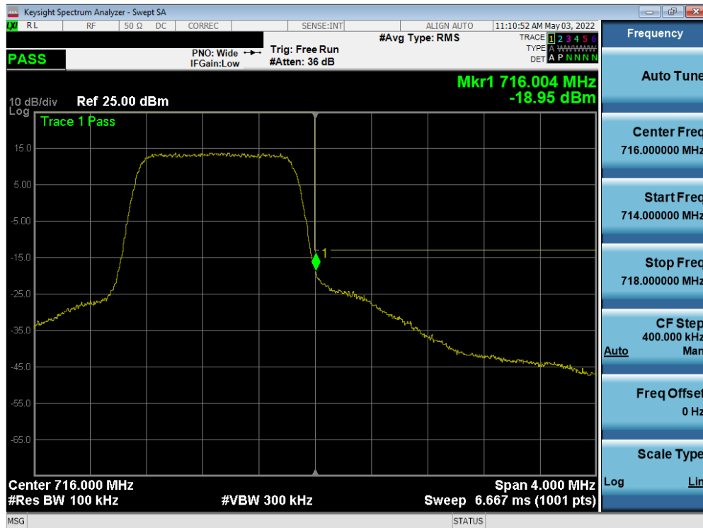
Plot 7-105. Upper Band Edge Plot (LTE Band 12 – 1.4MHz QPSK – Full RB)
