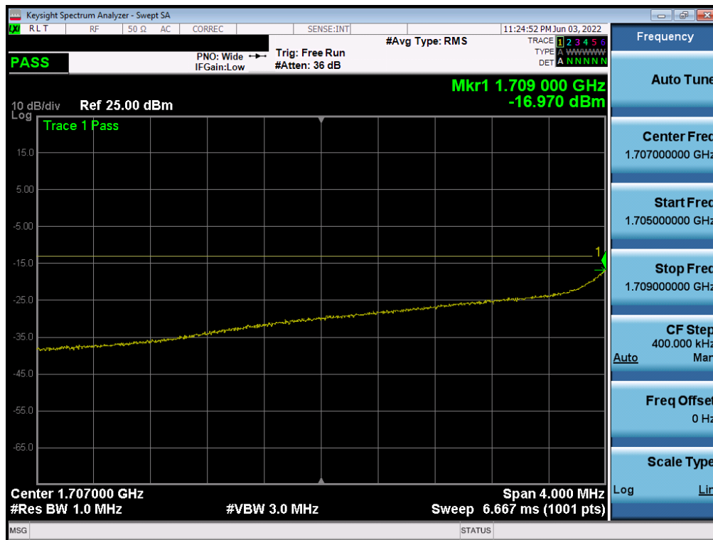
Plot 7-125. Lower Extended Band Edge Plot (WCDMA AWS – Ch. 1312)
