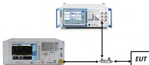
Figure 7-4. Test Instrument & Measurement Setup
