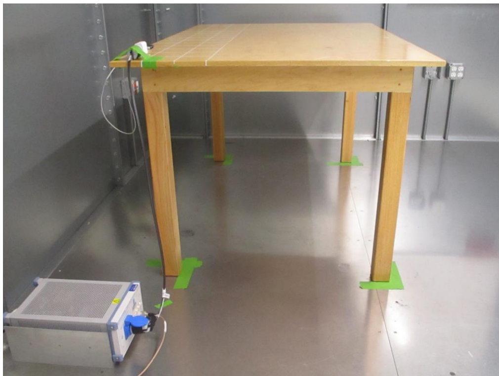
Figure 2: AC Line Conducted Emissions (Side View)
