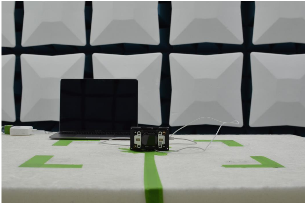
Figure 17: 30MHz-1GHz Test Setup (Rear View)
