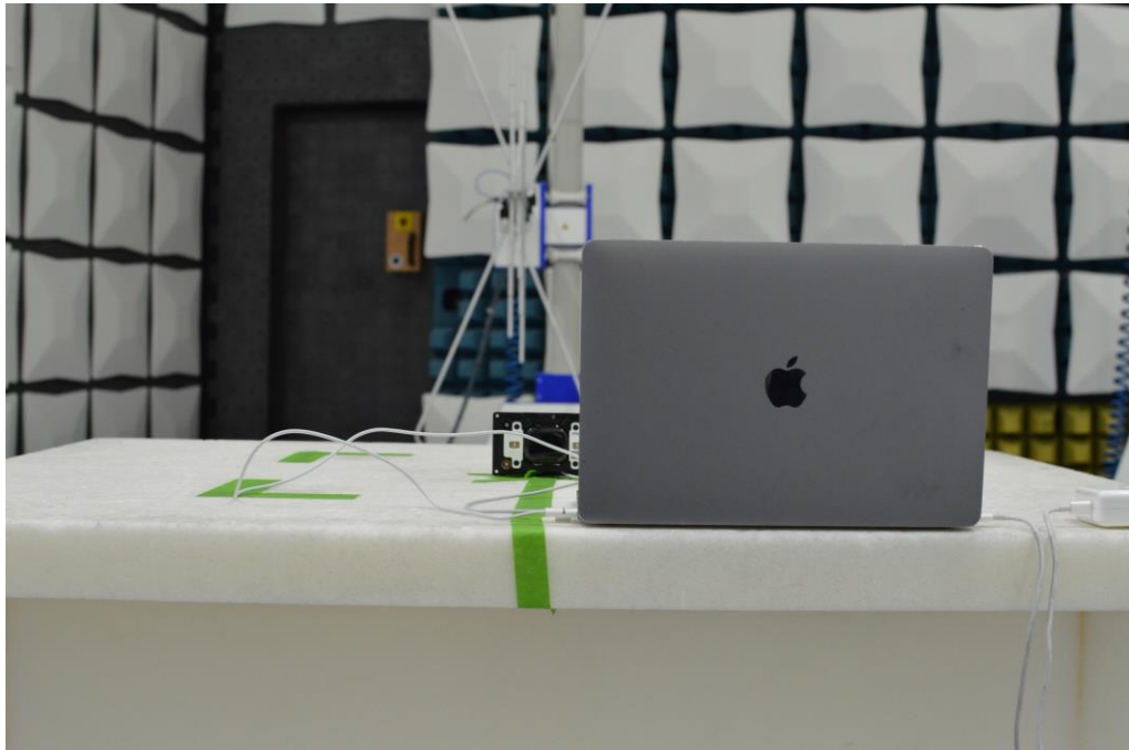
Figure 15: 30MHz-1GHz Test Setup (Rear View)
