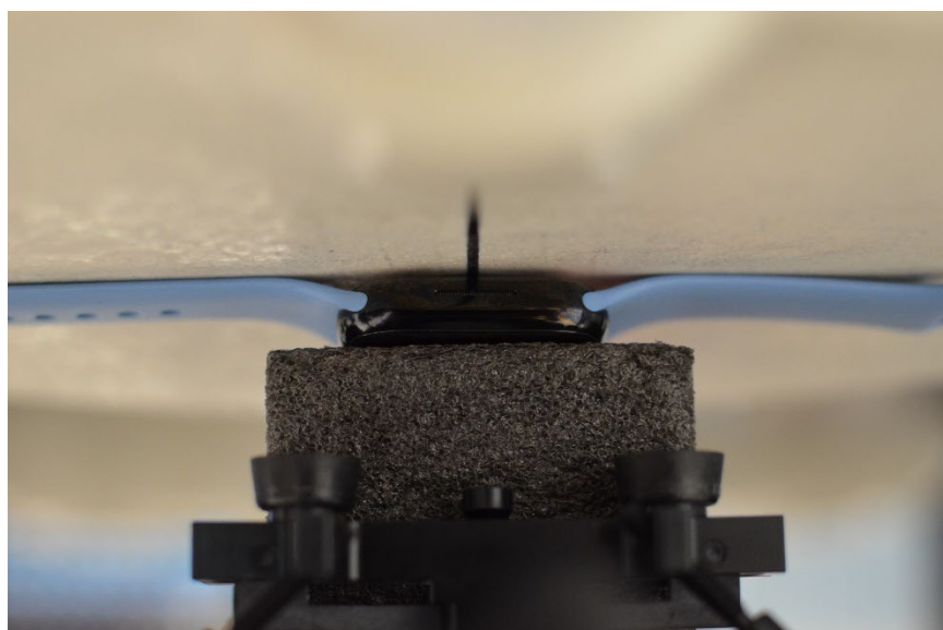
SAR Test Setup Photo 10: Stainless Steel with Sport Wristband, Extremity, Back Side at 0.0 cm
