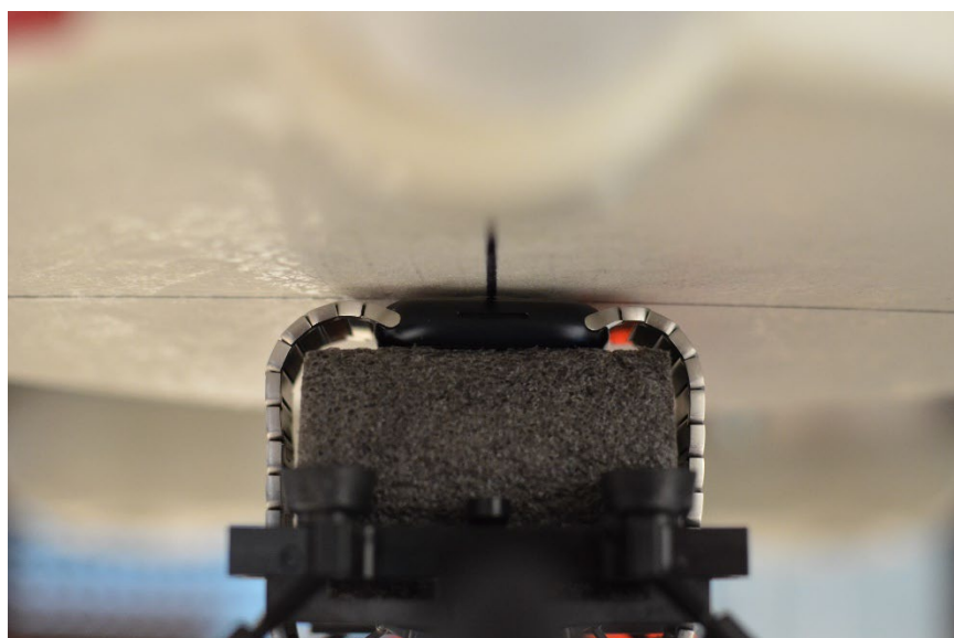
SAR Test Setup Photo 8: Aluminum with Metal Links Wristband, Extremity, Back Side at 0.0 cm
