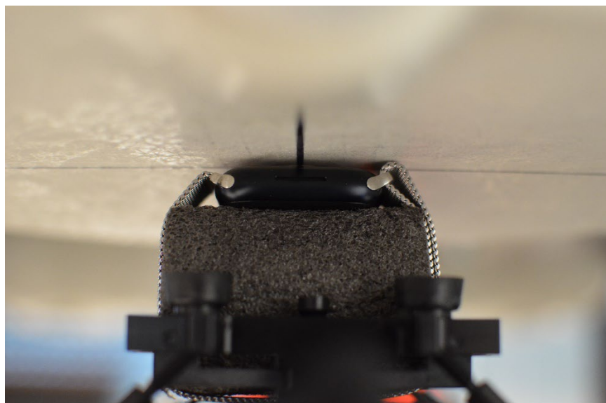
SAR Test Setup Photo 9: Aluminum with Metal Loop Wristband, Extremity, Back Side at 0.0 cm
