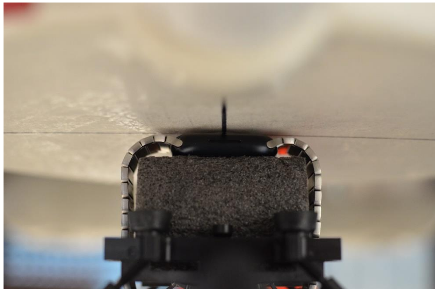
SAR Test Setup Photo 11: Aluminum with Metal Links Wristband, Extremity, Back Side at 0.0 cm
