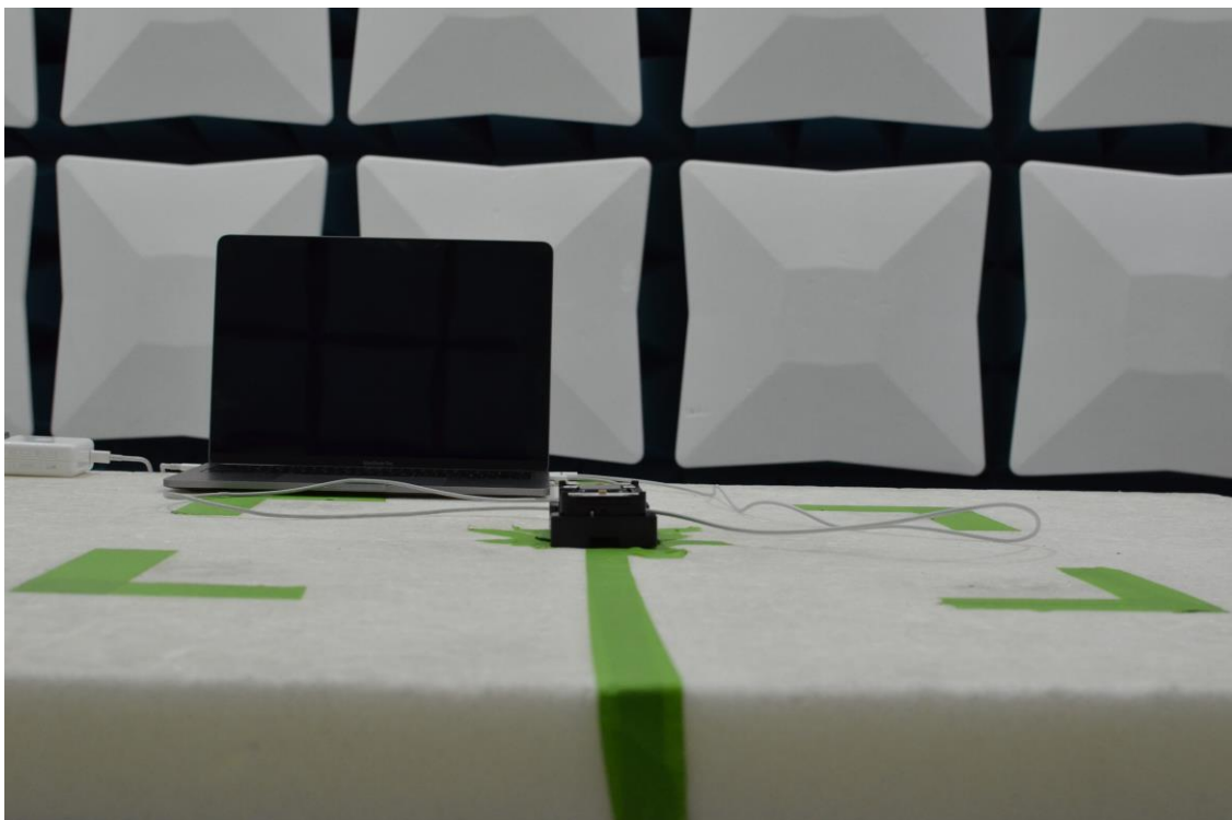
Figure 12: 30MHz-1GHz Test Setup (Front View)
