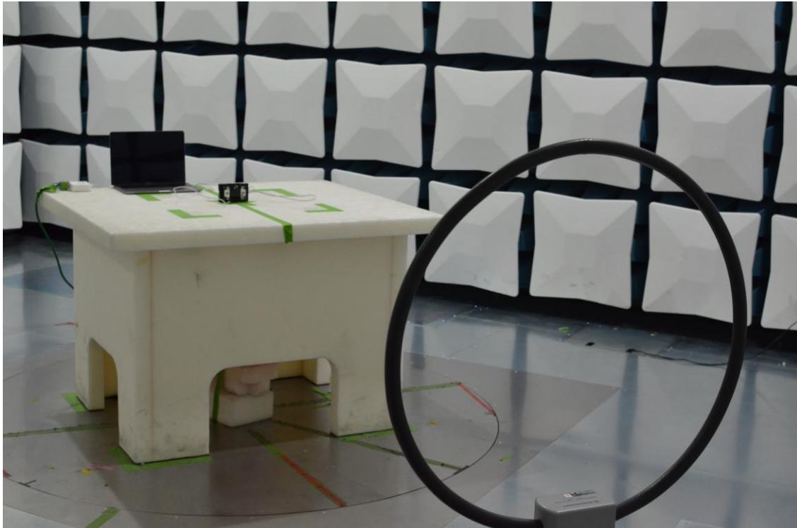
Figure 19: 9kHz-30MHz Test Setup (Front View)
