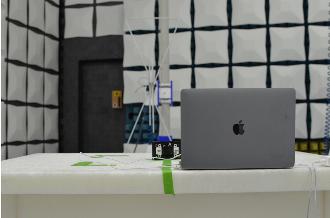
Figure 15: 30MHz-1GHz Test Setup (Rear View)
