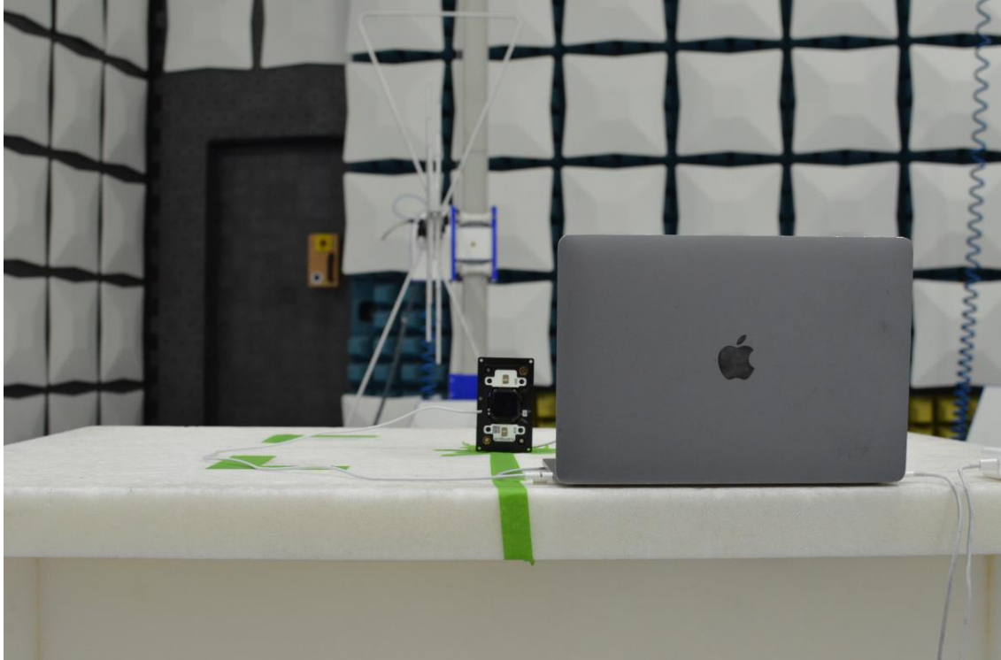
Figure 17: 30MHz-1GHz Test Setup (Rear View)
