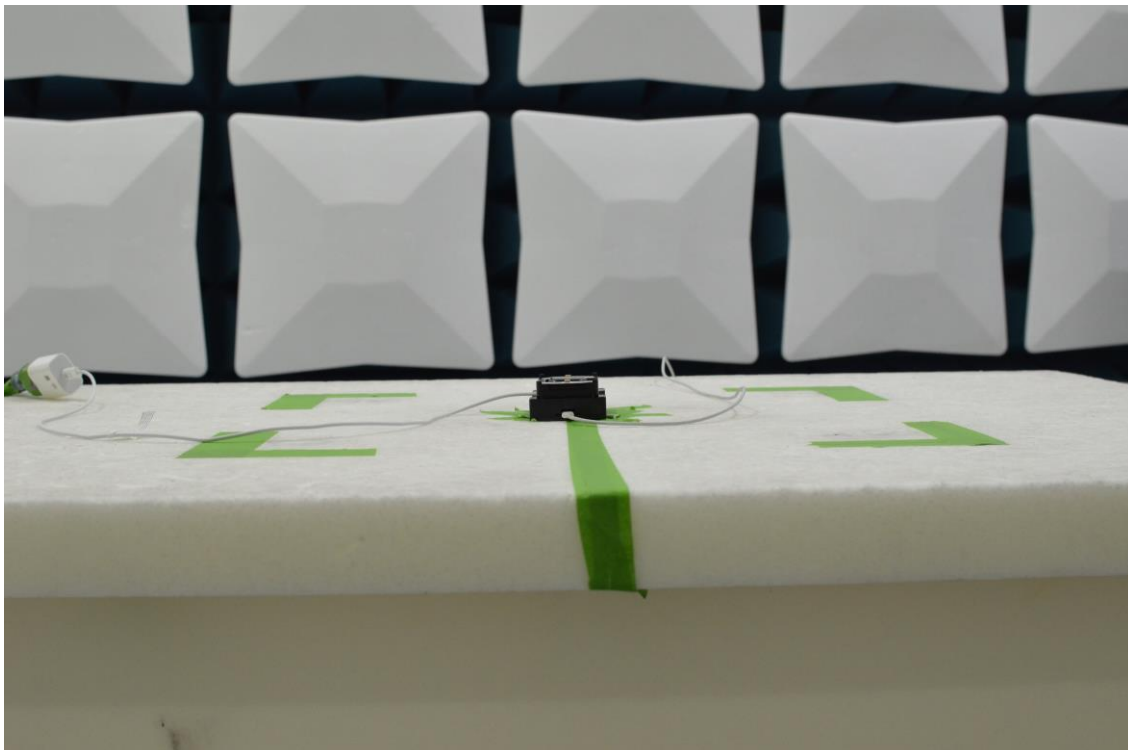
Figure 6: 1-18GHz Test Setup (Front View)
